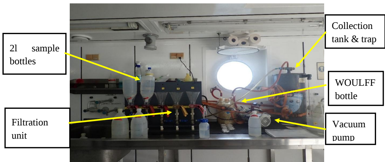
Fig. 5.7 The multi-unit vacuum filtration system used for suspended particulate matter sampling, including the filtration units, membrane pump, collection tank, and WOULFF bottle water trap.
