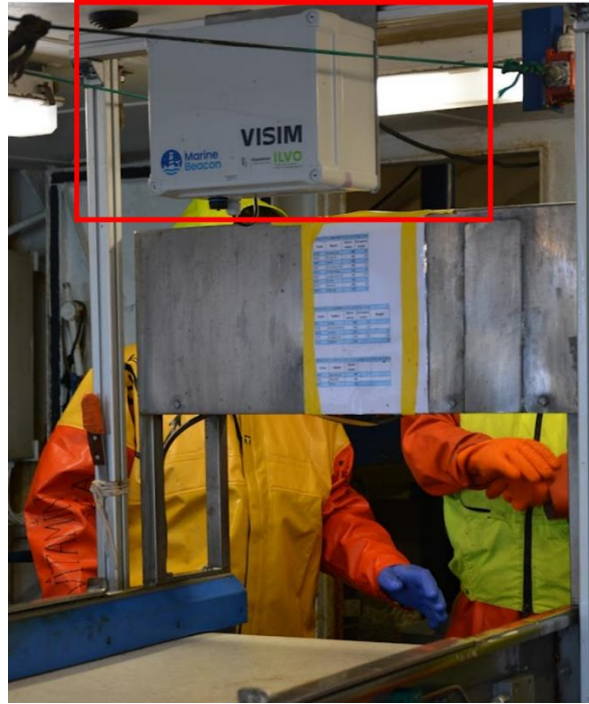
Figure 6-3 VISIM camera installed on the survey vessel during the NoriVis survey (red).
