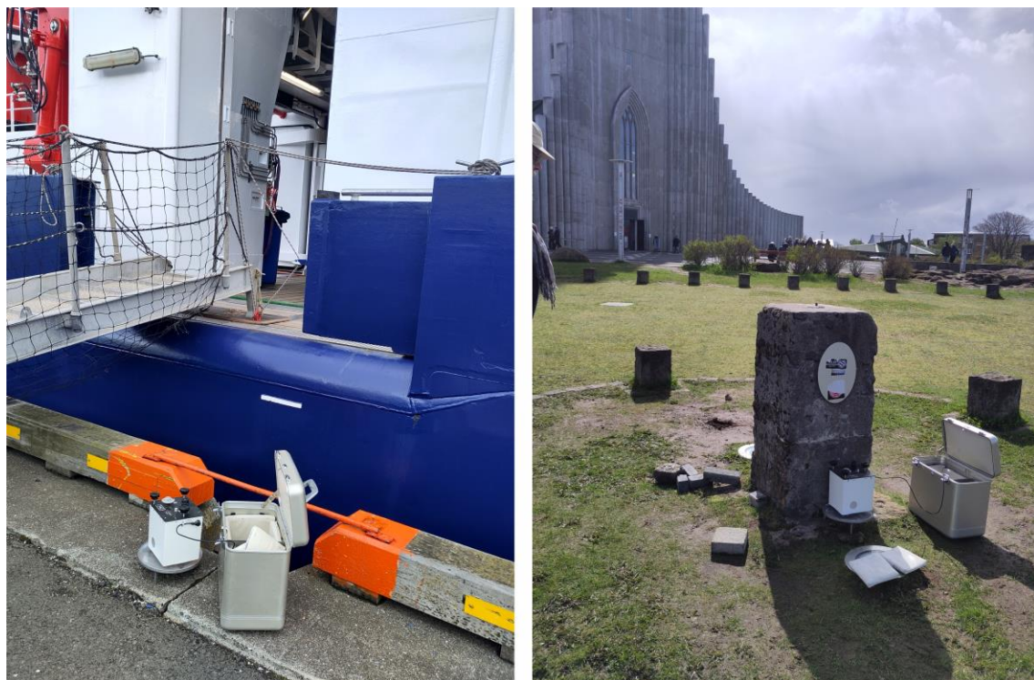
Fig. 11.7.4 Gravity measurement at the vessel before leaving (left) and at the reference station RVIK B near Hallgrímskirkja (right) in Reykjavik.
