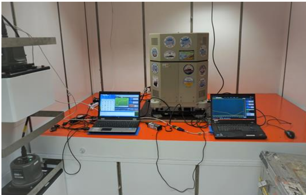
Fig. 11.7.2 KSS32-M gravimeter system mounted in the Gravimeter Lab on RV MARIA S. MERIAN.
