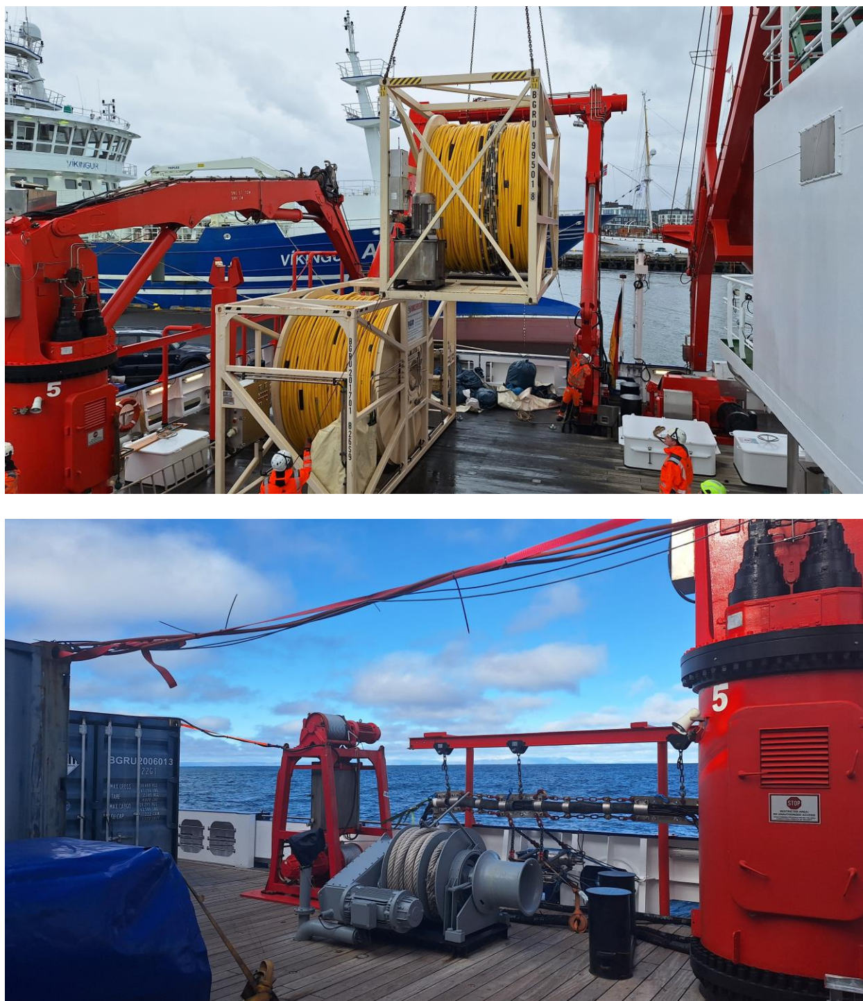
Fig. 11.1.1 Winches for seismic streamer (top) and air gun umbilical (bottom).
