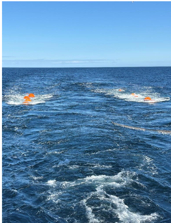
Fig. 11.3.2 Rear view from the vessel with port side and starboard side airgun arrays (orange buoys) and in the center the lead-in of the streamer cable. During acquisition, the lead-in was fixed with a cable-grip close to the sea surface.
