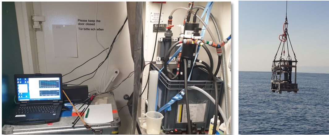
Fig. 4.2: Left: Continuous measurements of the extinction and absorption of light in Arctic surface waters using a AC-S (Seabird) mounted to Polarstern's surface seawater pump system. From those measurements directly, the absorption and scattering of particles and CDOM is determined for the whole spectrum in the visible resolved with about 3 nm resolution. This data then can be decomposed various specific algorithms to determine the particle size distribution and the various phytoplankton pigment composition. Right: Underwater light field measurements with TRIOS RAMSES radiometers detecting the hyperspectral up- and downwelling radiation and the AC-S (Seabird, including pressure sensor, data logger and battery) measuring extinction and absorption.
