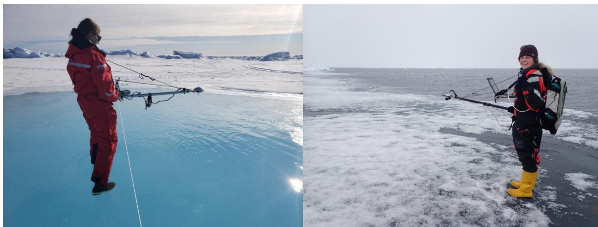
Fig. 2.1.1: Left: A Kipp and Zonen albedometer was used to measure broadband albedo, photo from 22 July 2025 on R3a. Right: An ASD FieldSpec3 spectroradiometer was used to measure spectral albedo, photo from 1 August 2025 on R2b.
