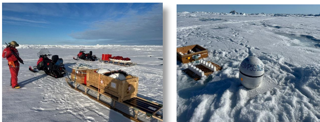
Fig. 4.9.2: Recovery and deployment of the CTD buoys. Left: Transport of the equipment and buoy on a Nansen sled with skidoos. Right: CTD buoy after deployment on sea ice. Photos: Jacob Allerholt
