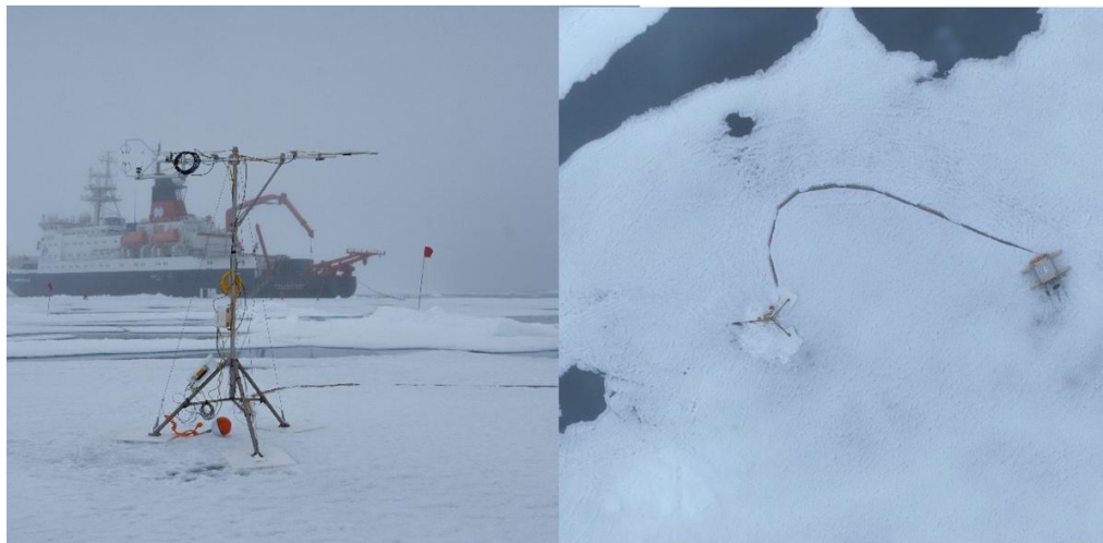
Fig. 3.3.3: Left photo: SEB tower after deployment at ice stations 2a – Florian Gebhardt/DE.AWI. The CNR4 net radiation sensor is pointing to the right. The tower was surrounded by melt ponds but was standing on thick ice. Right photo: a drone picture during ice station 2b – Sandro Dahlke/DE.AWI. The melt pond had deepened and extended towards the tower. At the bottom left there was an elevated spot of about half a meter height. The larger area was also dominated by melt ponds, but also medium-sized ridges as seen in Figure 3.3.1 (center).
