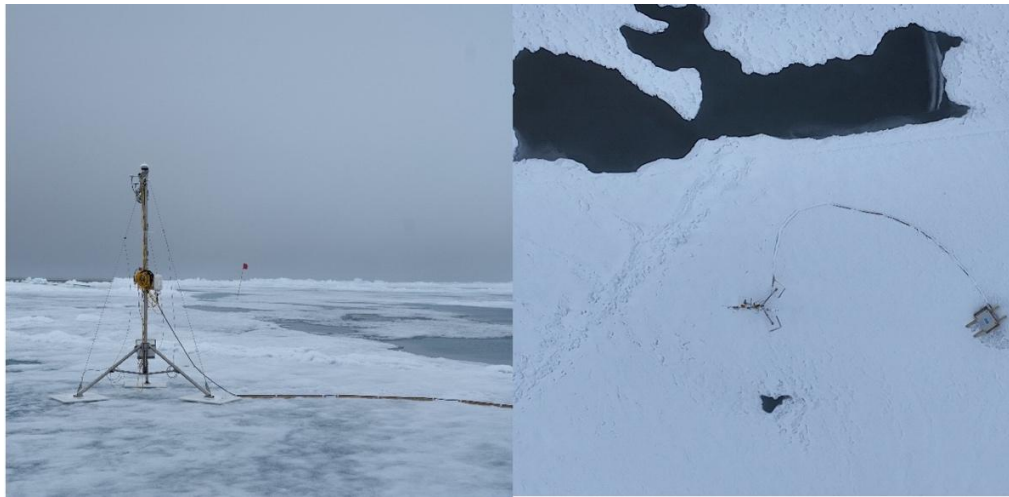
Fig. 3.3.2: Left photo: SEB tower after deployment at ice stations 1a – Florian Gebhardt/DE.AWI. The CNR4 net radiation sensor is facing the camera. The tower was located next to a refrozen lead (right) including some ponds and a small ridge (behind the tower). The area was dominated by flat undeformed first-year ice. Right photo: a drone picture during ice station 1b – Sandro Dahlke/DE.AWI. The small ridge is visible on the right-hand side, while the ice surface had brightened and the ponds inside the refrozen lead had deepened.
