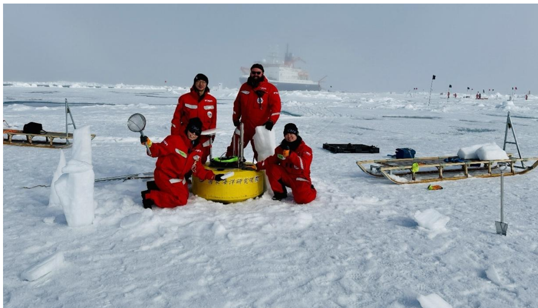
Fig. 4.4.7: Deployment of NAMR surface buoy system equipped with a GPS beacon a dual GPS antenna and a downward-looking Nortek Signature 250 kHz ADCP
