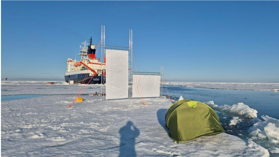
Fig. 3.5.2: Screen setup at the lead of station 1c. The wind blows from the ocean on the right over the ice. The thermal infrared camera pointing at the synthetic screens is shielded from direct radiation by the green tent. Photo: Michael Haugeneder/CH.WSL
