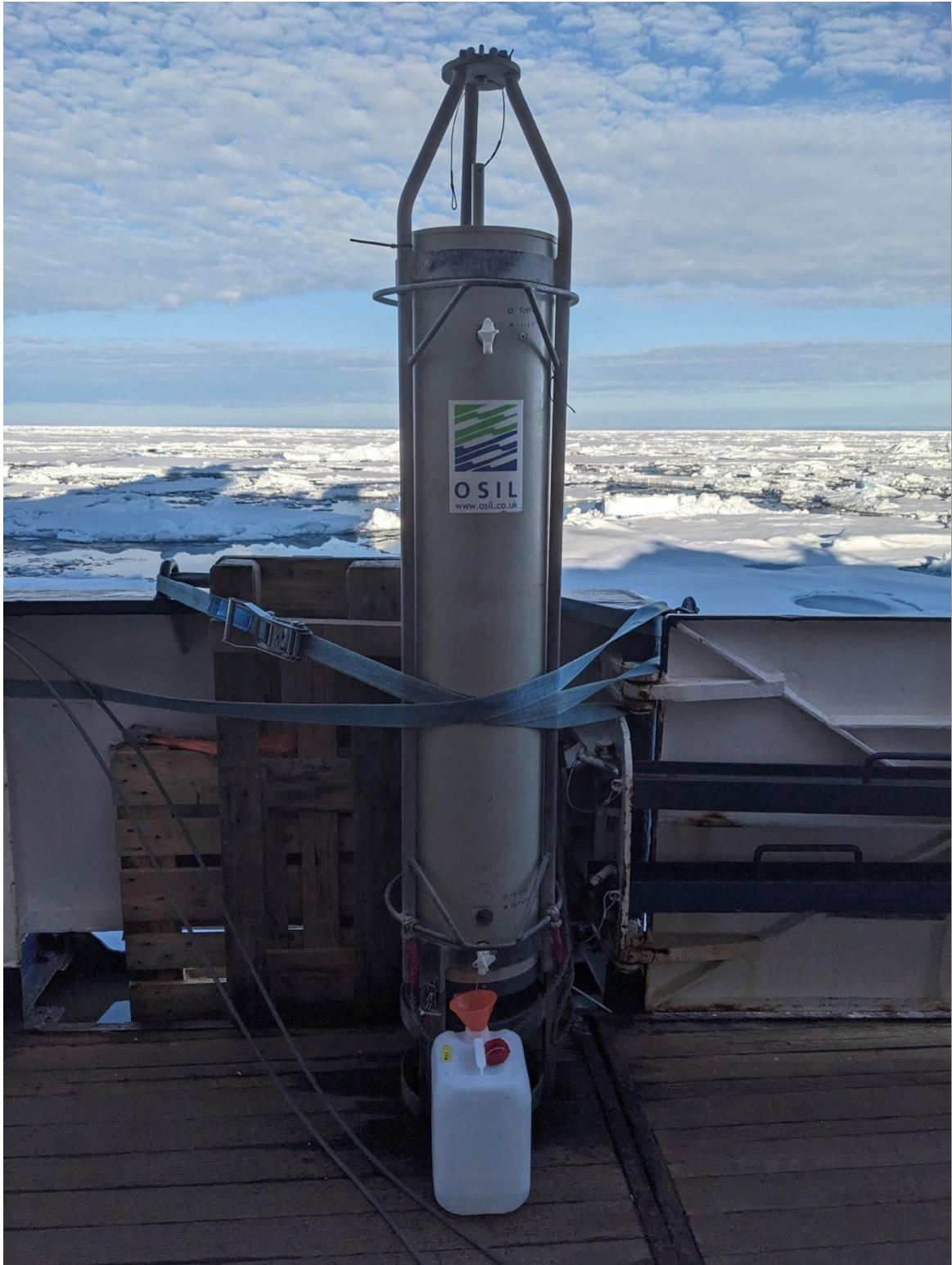
Fig. 5.5.9: Marine Snow Catcher during deployment at PS149. The Marine Snow Catcher collects intact settling aggregates, allowing for direct measurements of aggregate size-specific settling velocity and microbial respiration on board. Picture taken by Runa Reuter
