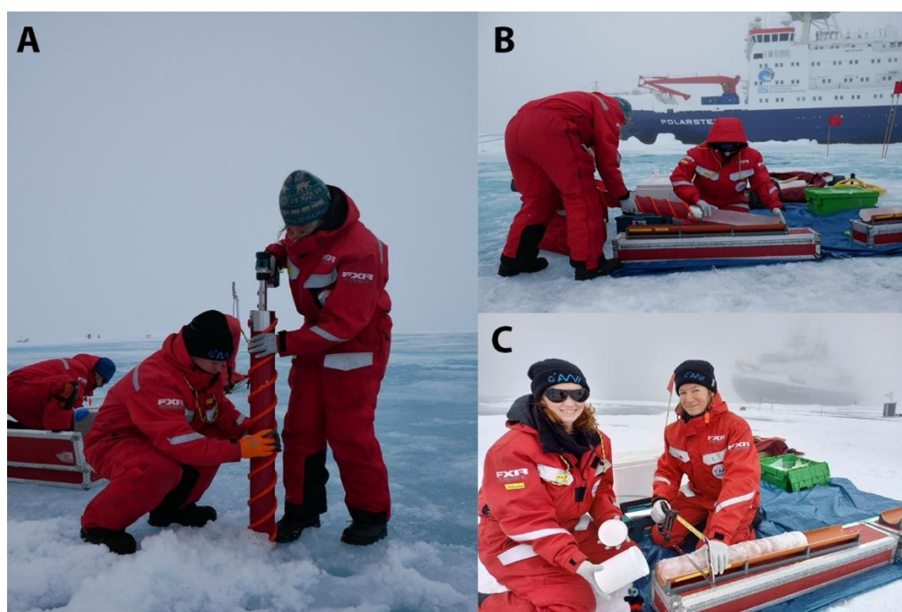
Fig. 5.1.1: Images of ice-core sampling procedure. A) Ice-core sampling using the Kovacs Corer (9 cm). B) Placing the ice-core into the half pipe for length determination. C) Dividing the ice core into the three sections; bottom 10 cm, middle part (10 cm to 50 cm), and the top part (from 50 cm to the surface). Picture credits: A) Julia Wenzel (DWD), B) Julia Wenzel (DWD), Lena Eggers (AWI).
