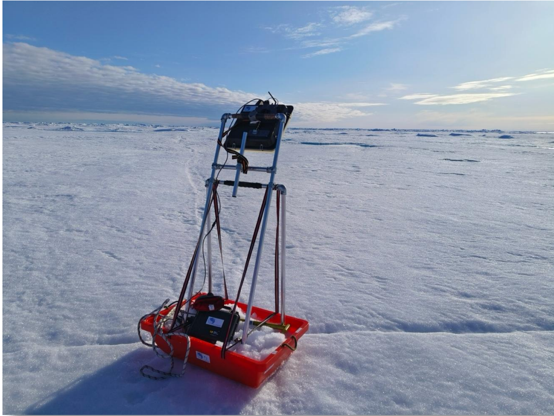
Fig.2.6.1: ARIEL deployed on a plastic sled during ice station work, measuring a homogeneous ice surface
