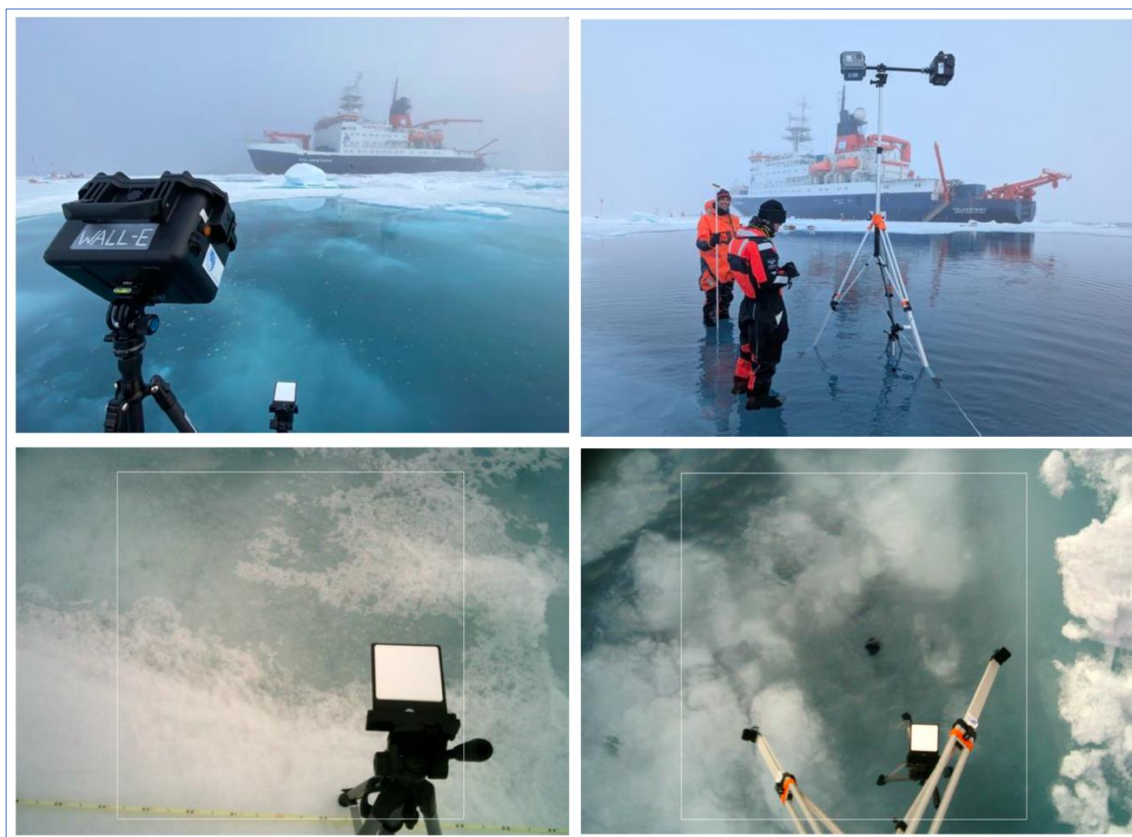
Fig. 2.5.1: Examples for the two different camera set ups. Left images: Transect measurement on small tripod with 40° incidence angle. Right images: Nadir pond measurement (90° incidence angle) with co-located drill hole in the image center. The white square marks the extend of the hyperspectral measurement. The white plate is the white reference.
