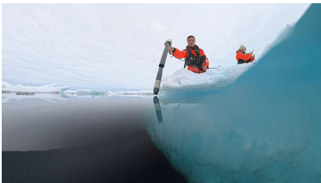
Fig. 4.3.1: An XCTD was deployed along the lead edge of ice floe. Photo credit: Ke-Hsien Fu
