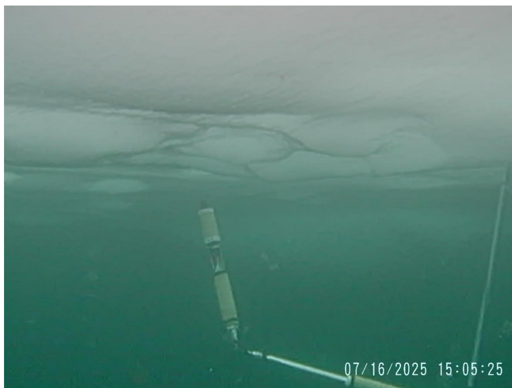
Fig. 4.7.1: Underwater photo of L-arm deployment. The radiometer is on the left side of the image and is pointing upwards at the ice bottom. In this case, the radiometer is not fully vertical due to it being dragged by the drift. Subsequent modifications of the floatation resolved this issue.
