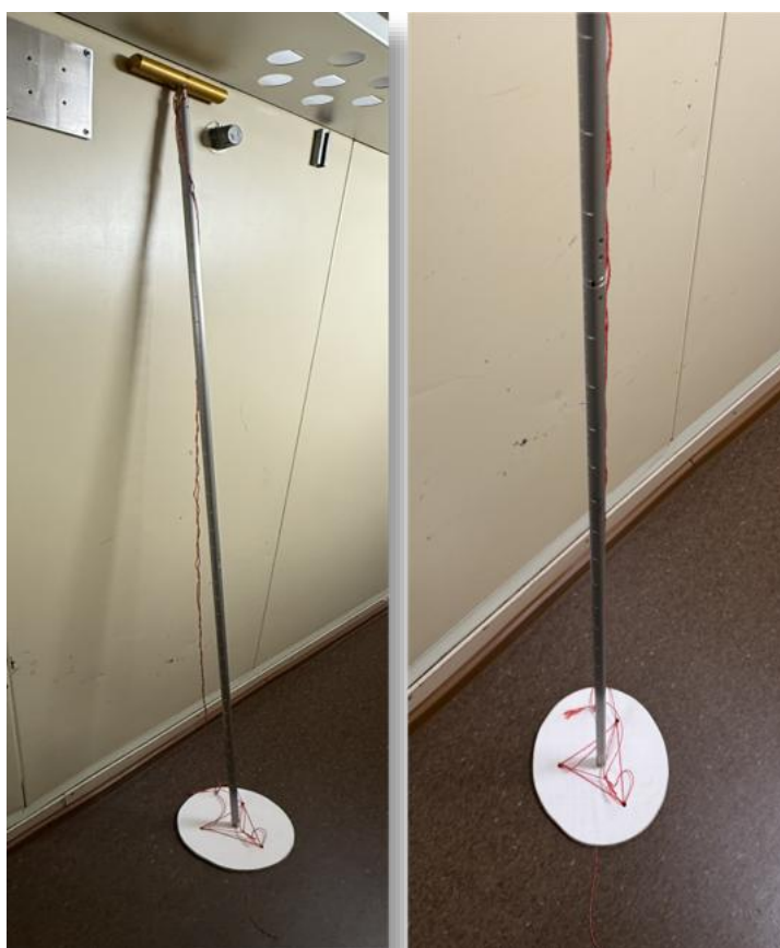
Fig. 2.7.1: Image of the Snow Probe. A wooden plate is attached to minimize pond bottom penetration. The primary objective was the validation of bathymetry measurements from airborne sensors and the assessment of temporal changes in melt pond depth. For a consistent comparison of the measurements, cross-sections obtained with the folding meter, MagnaProbe, and Snow
