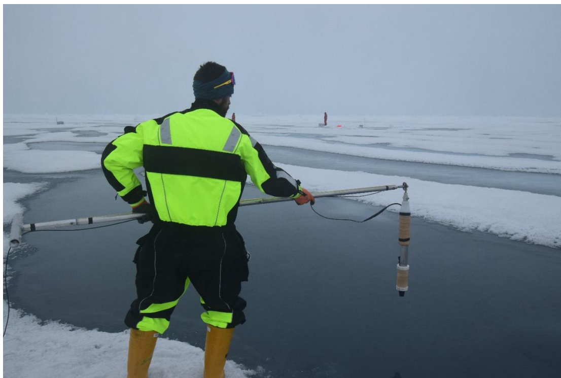
Fig. 4.7.2: Photo of using the L-arm to measure albedo of a pond. The sensor was held approximately 25 cm above the surface.
