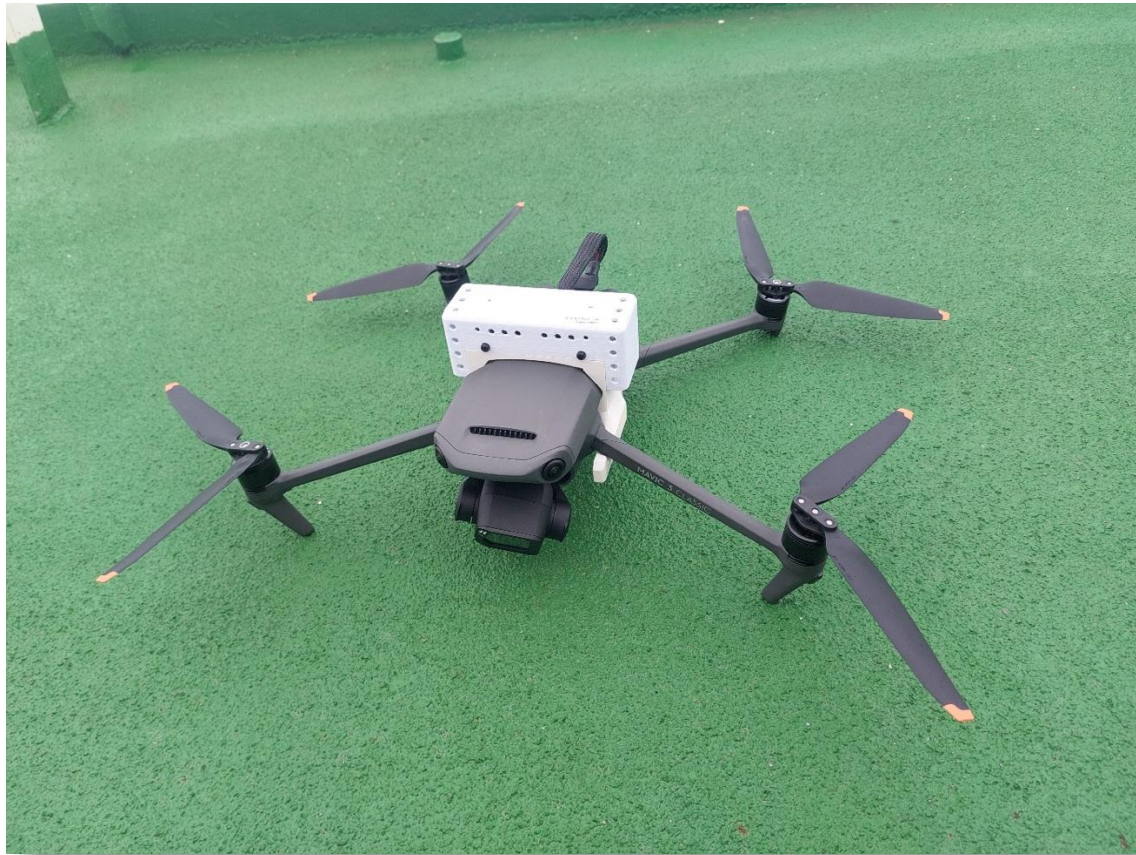
Fig. 3.1.2: DJI Mavic 3 Classic drone equipped with a backpack for meteorological measurements. Photo: Sandro Dahlke/DE.AWI
