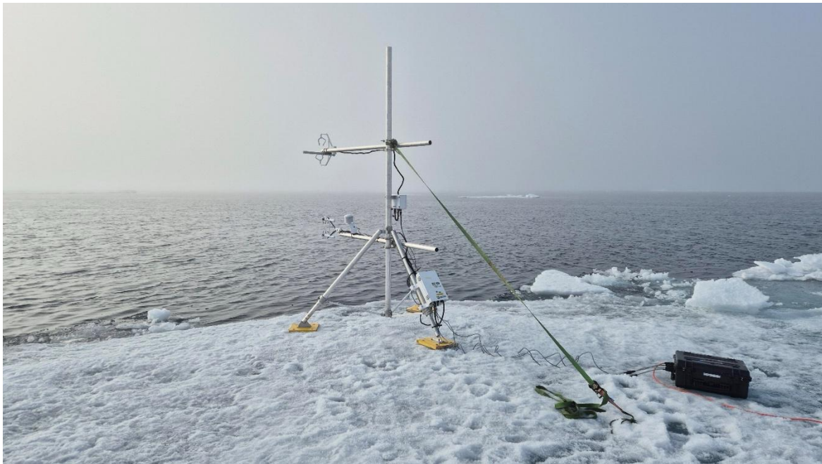
Fig. 3.5.1: Flux tower at the transition from lead to sea ice with an IRGASON at 1 m height and a CSAT3 at 2 m above the sea. Setup at station 1c. Photo: Michael Haugeneder/CH.WSL
