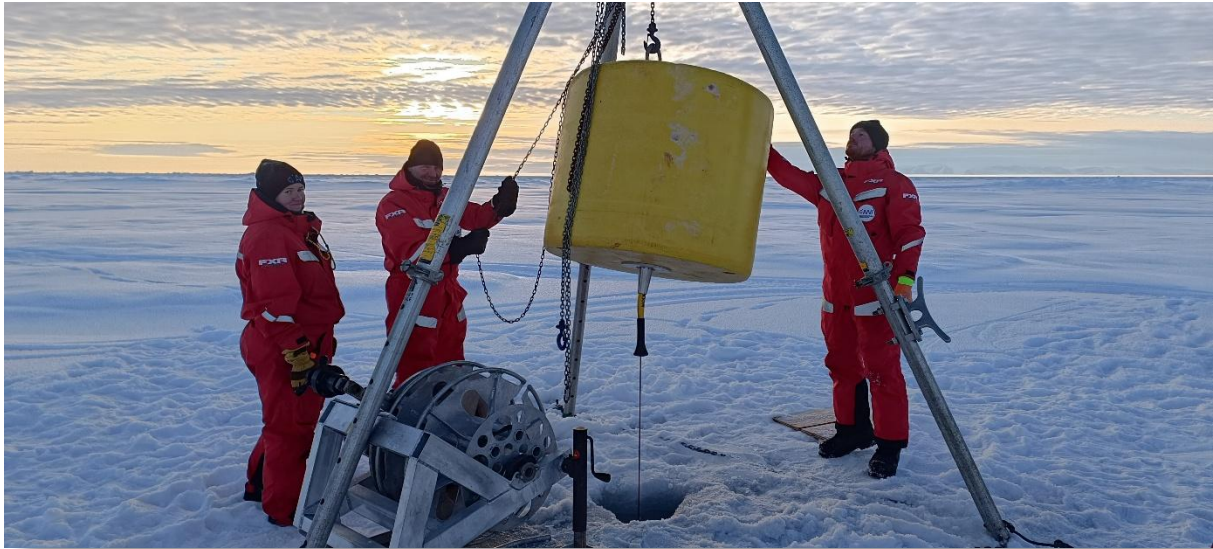
Fig. 2.33: Lifting the surface unit and the floatation package on top of the hole. Photo by Mario Hoppmann.
