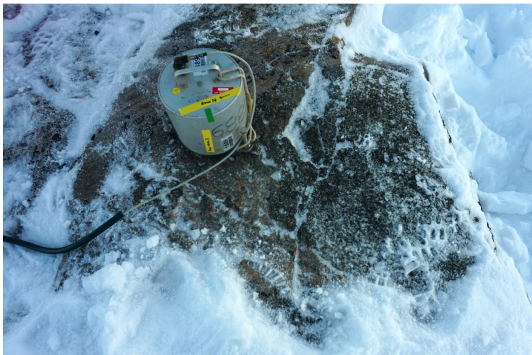
Fig. 5.1.3: Seismometer installed on bedrock
