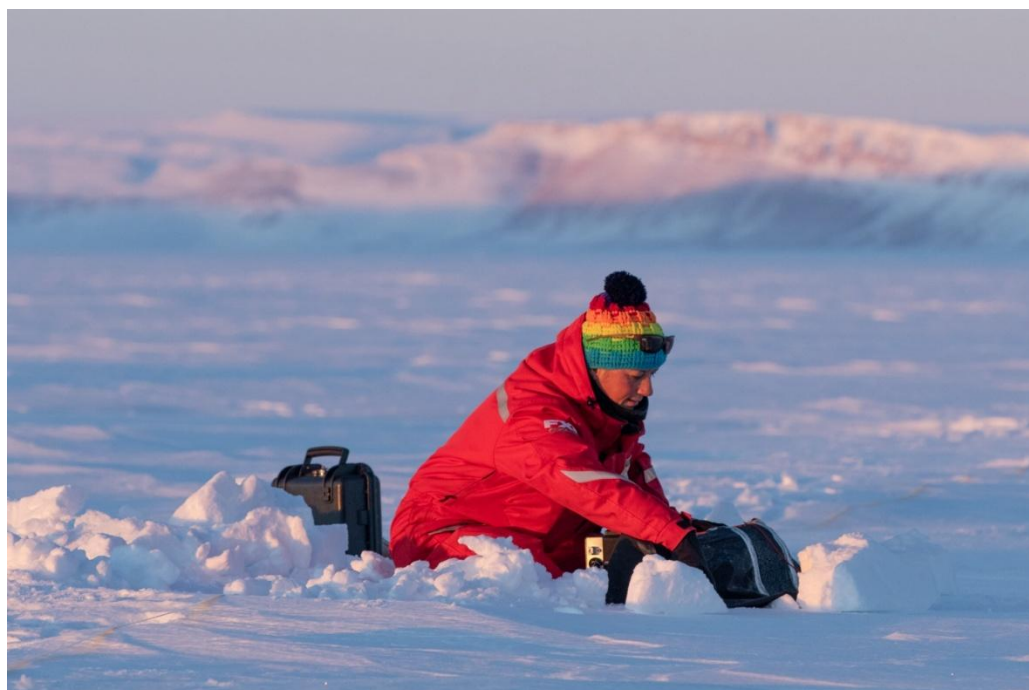
Fig. 4.7.1: SnowImager measurement of a snow pit wall (Photo: Marcel Nicolaus, AWI)
