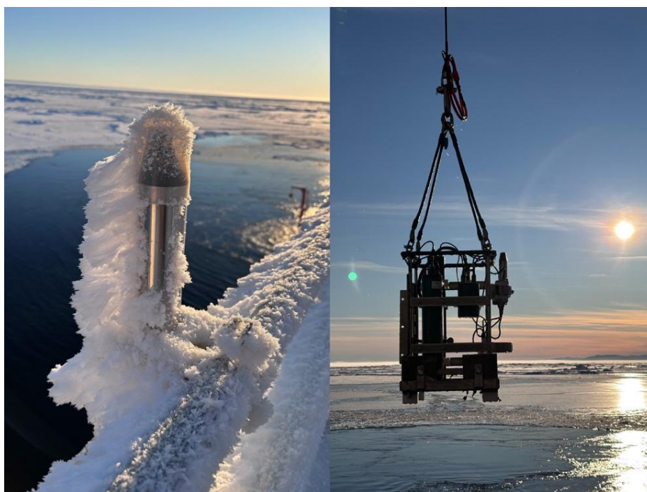
Fig. 3.4: RAMES radiometer sensor mounted above Deck A to measure the sunlight irradiance (left) and the light profiler (right)
