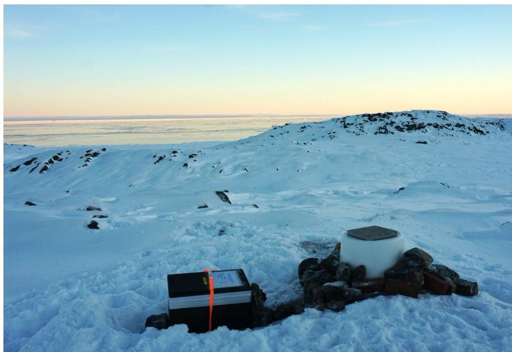
Fig. 5.1.4: Fully mounted seismic station on land. The seismometer is covered by the bucket, data recorder and battery supply are contained in the insulation box.
