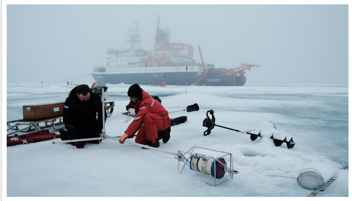
Fig. 4.15: Setup of the RDI 300kHz ADCP to complement the MSS measurements. Photo credit: Mario Hoppmann
