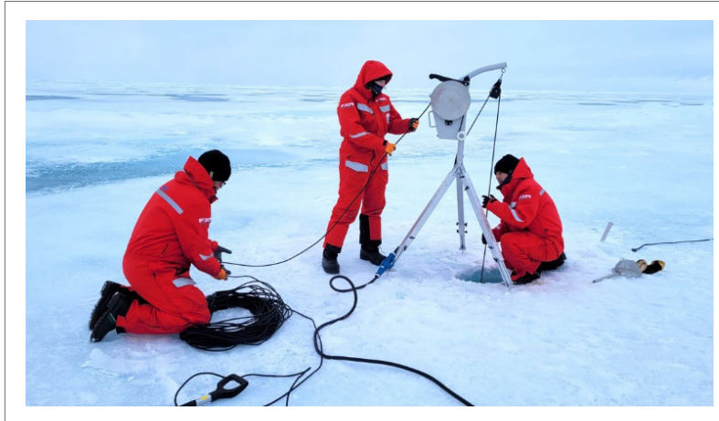
Fig. 7.18: Recovery of longlines using an electrical line hauler (Northlift LH 300). Photo: Magnus Lucassen
