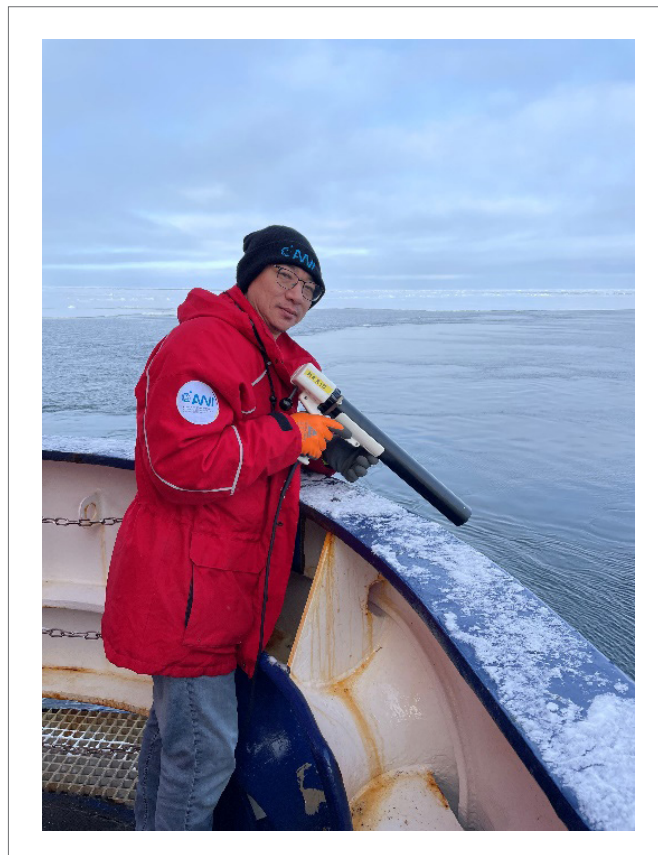
Fig. 4.3: XCTD deployment using a hand-held launcher from the aft of the ship; photo credit: Jialiang Zhu
