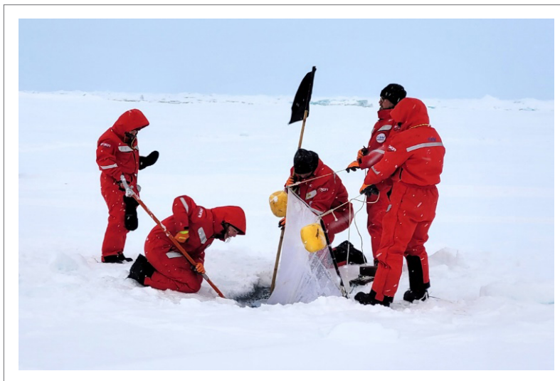
Fig. 7.19: Deployment of the fyke net under ice. Photo: Magnus Lucassen
