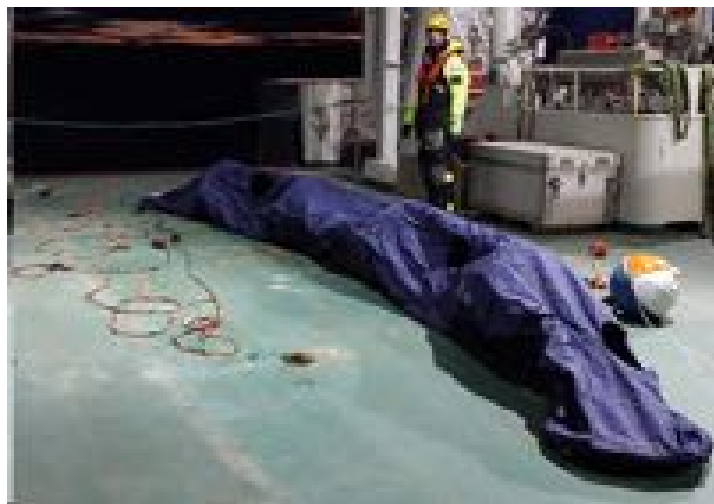
Figure 14: Deployment of a CMRE SVP drifter: surface buoy (blue-white-orange), drogue (blue) and hydrophone array (orange/black cables and black hydrophones and pressure-temperature sensors).
