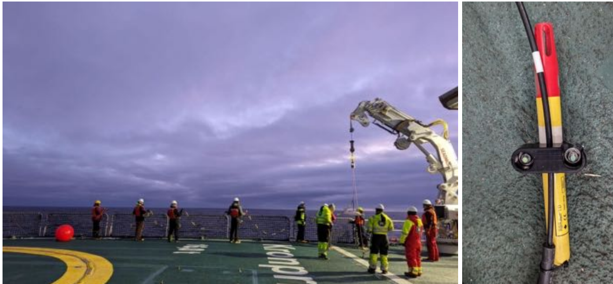
Figure 7: Left: Deployment of the bow chain from the starboard side of the ship, The line of thermistors is lowered by the science crew as the 200lb weight is lowered by the winch and the ship's knuckle crane. Right: an example of the thermistor attached to the line. The line was 30m long with 59 thermistors attached every 0.5 m.
