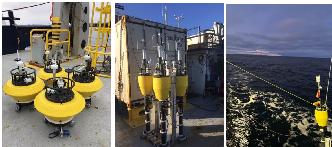
Figure 16: version 4 (left) and version 3 (right) SWIFT buoys. The v3 buoys include a small heave plate and hydrophone hanging 15 m below the buoy.
