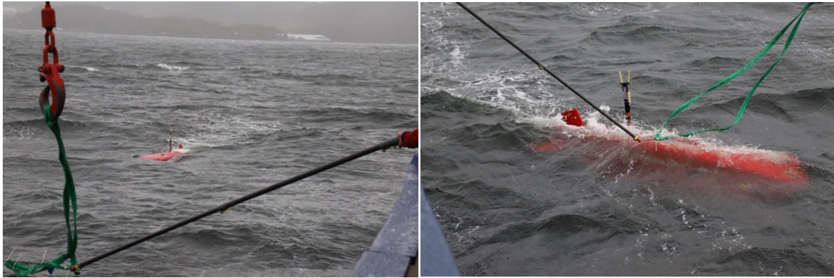
Fig. 6.2: Left image shows IMGAM AUV approaching RV Heincke for recovery. Right image shows the AUV getting hooked for the recovery.
