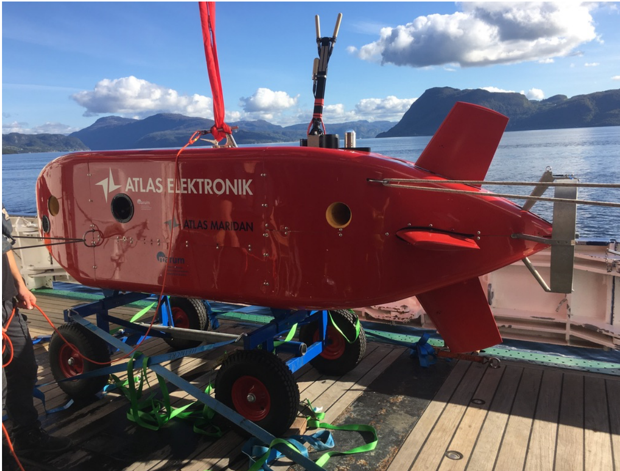
Fig. 6.1: IMGAM AUV on its deployment cart on board RV Heincke.
