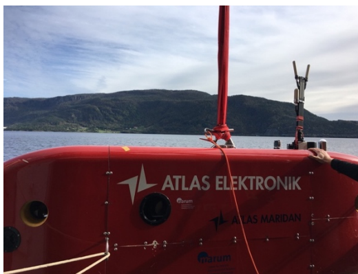
Fig. 6.6: IMGAM AUV Penguin hook rigged for slip lifting.
