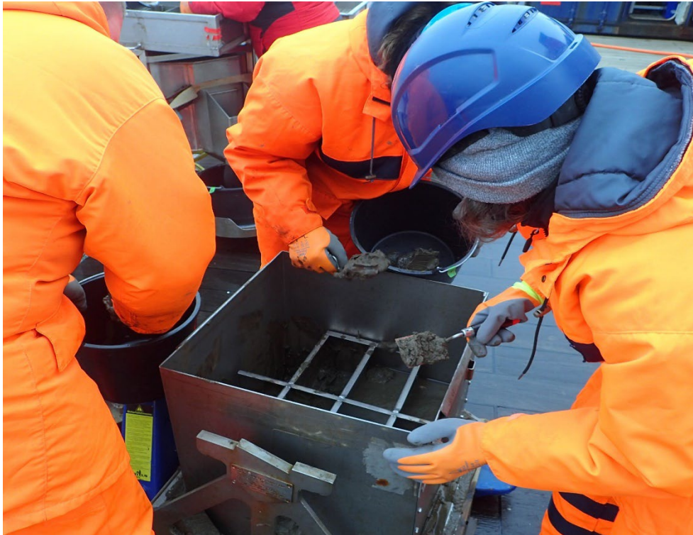
Fig. 5.2.3 Subsampling of the Giant Box Corer (GBC) after retrieval of the gear (Photo: J. Dannheim).
