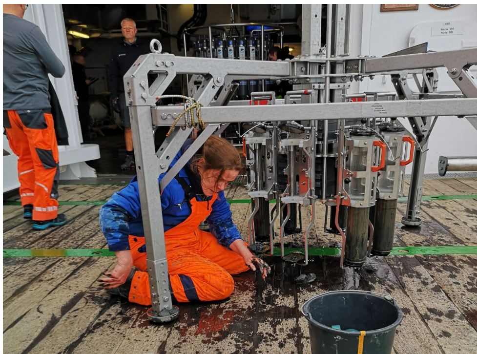
Fig. 5.2.1 Retrieval of sediment cores right after the recovery of the Multiple Corer, MUC (Photo: J. Schnier).
