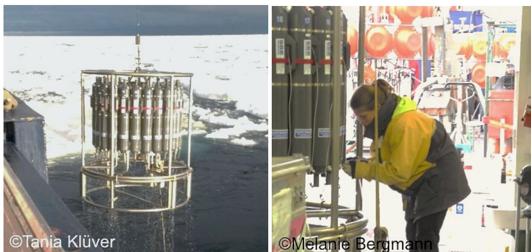
Fig. 5.1.1 Recovery of the CTD / Rosette Water Sampler (left) and water subsampling from the instrument's Niskin bottles (right).
