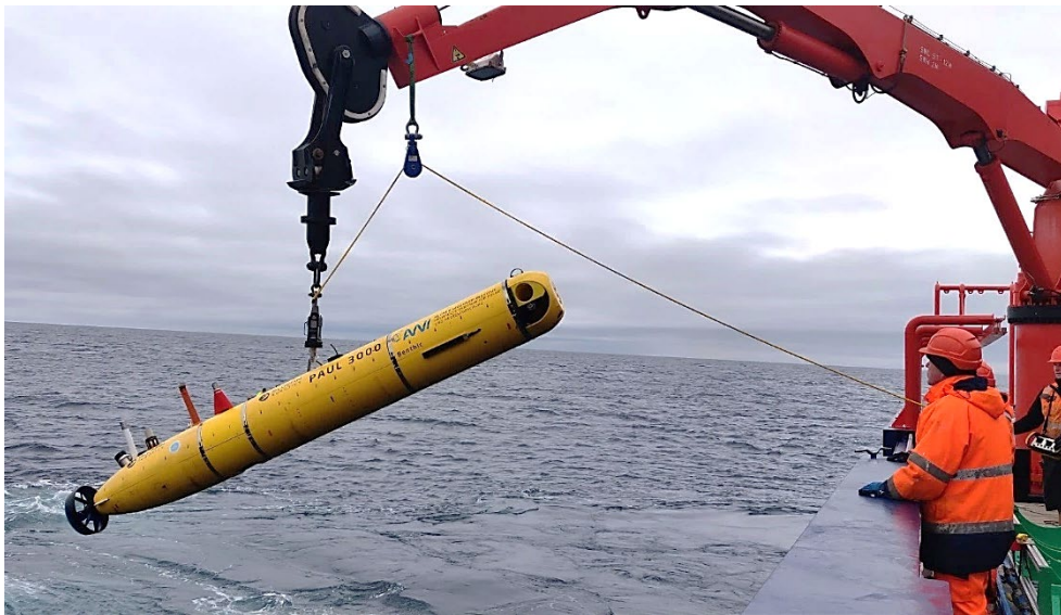
Fig. 5.3.1 Deployment of the Autonomous Underwater Vehicle (AUV) ‘Paul’ during expedition MSM108.
