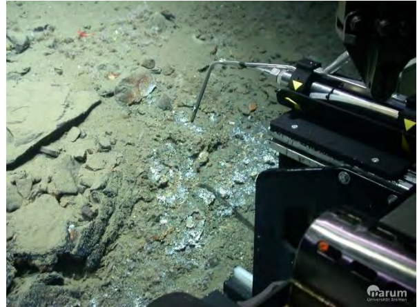
Fig. 5.8.18 Applying the temperature probe on the ROV did not measure any changes associated with the white patches / staining.
