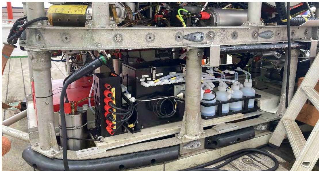
Fig. 5.8.59 The fluid sampling system KIPS deployed from MARUM ROV QUEST during MSM109.
