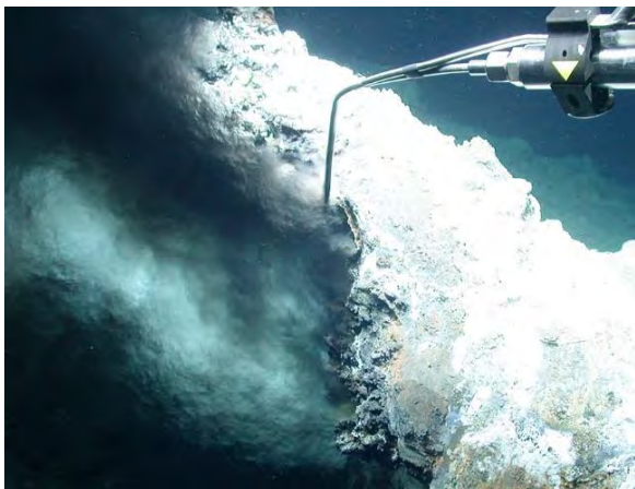
Fig. 5.8.43 Temperature probe measurement and fluid sampling at the Black Smoker
