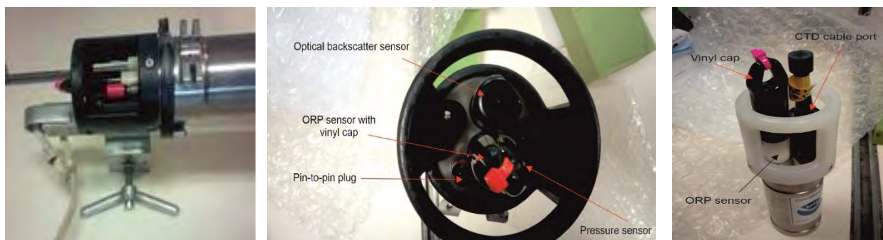
Fig. 5.4.1 (left): The non-autonomous ORP sensor attached to the CTD, (middle) top view of MAPR-74 showing all sensors, (right): MAPR-74 attached to the clamp device with metal rings
