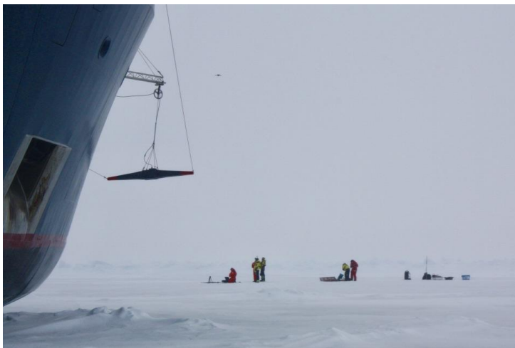
Figure 39 - The SIMS ElectroMagnetic sensor suspended from the front of the boat allows to real time measurements the total Sea Ice Thickness (including the snow). We can also guess the drone in front of the ship, at the level of the SIMS support beam.
