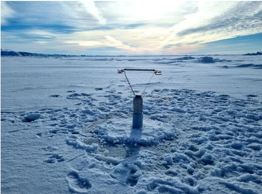
Figure 23 - Ice-T buoy with 120 GHz and 24 GHz snow radars mounted on top. Deployment in Baffin Bay offshore Upernavik, Greenland, on 31 March 2022 in 55 cm-thick sea ice underneath a Sentinel 3 ground-track.
