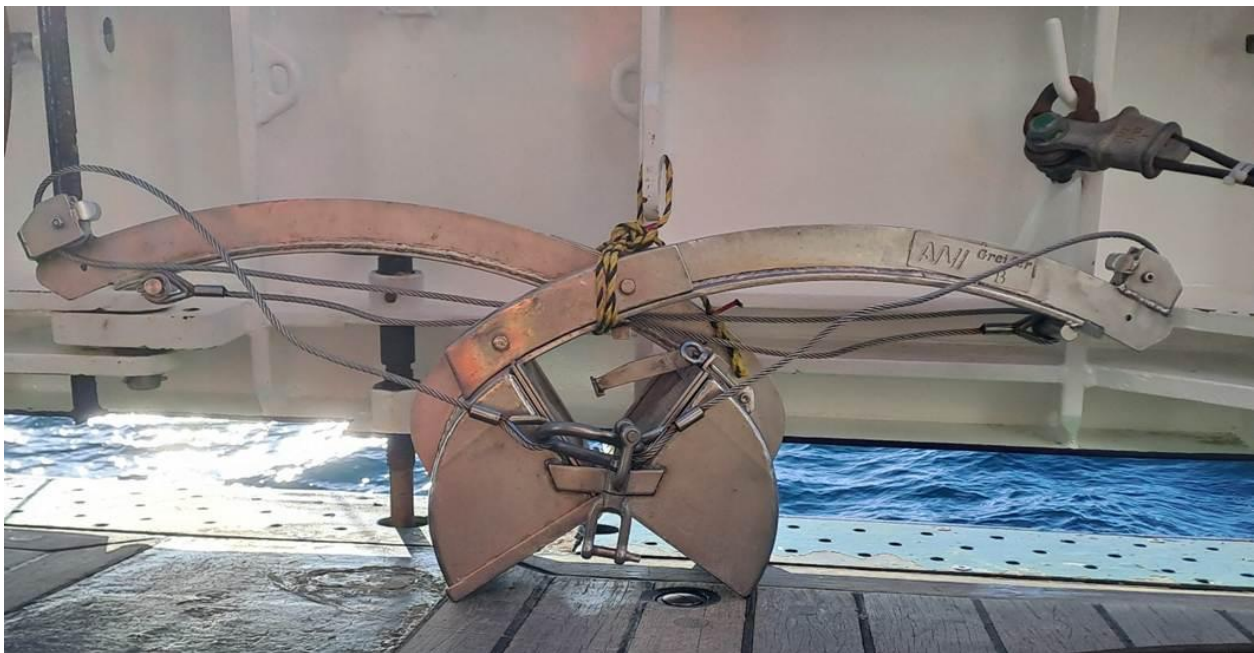
Fig. 5.16 The van-Veen-Grab on deck.
