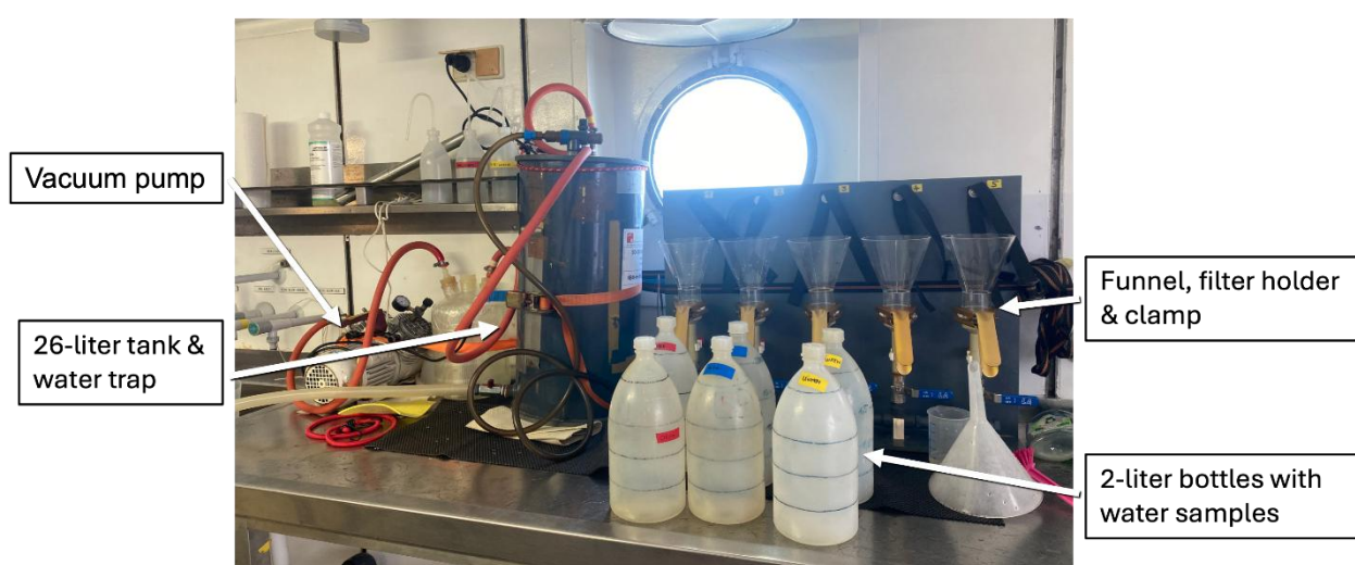
Fig. 5.7 Filtration set-up with the main components.
