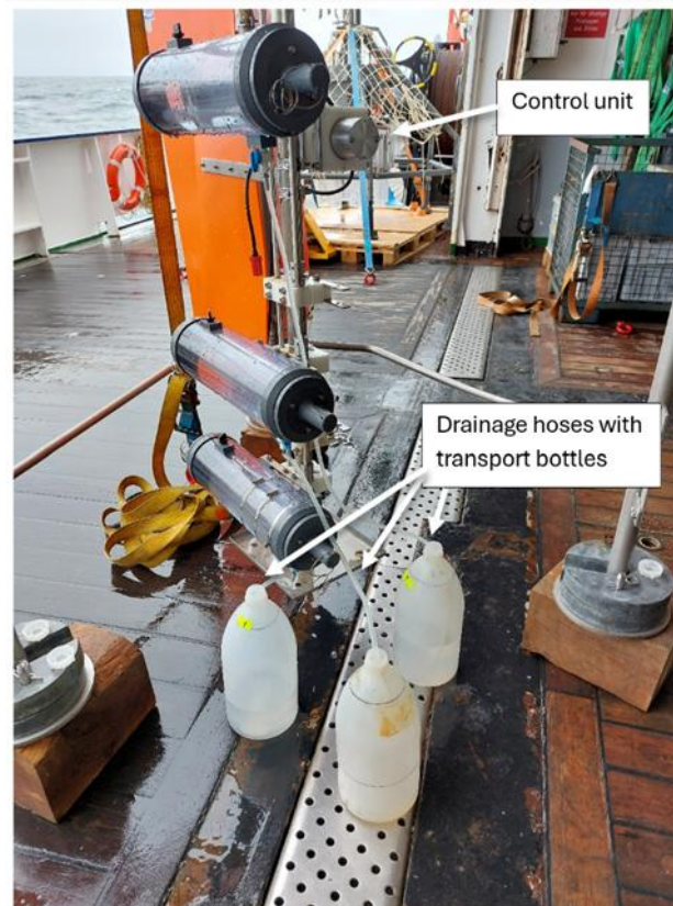
Fig. 5.13 Drainage of BWS NISKIN bottles.
