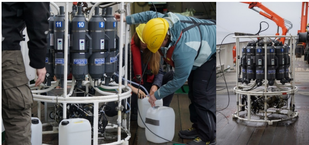
Fig 5.3.2 CTD at RV HEINCKE, before profile (right) and after profile (left), water samples collected in canisters.
