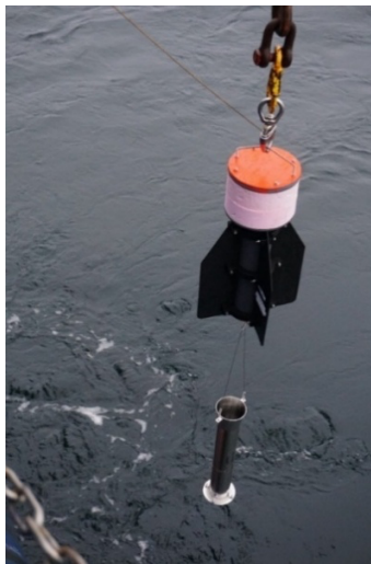
Fig. 5.9.2 Drifter with plastic trap during the deployment
