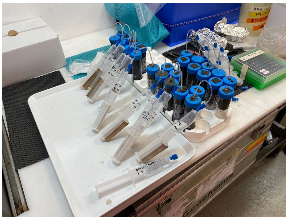
Fig. 5.10 Procedure of bottom water extraction using rhizone mounted on syringes.
