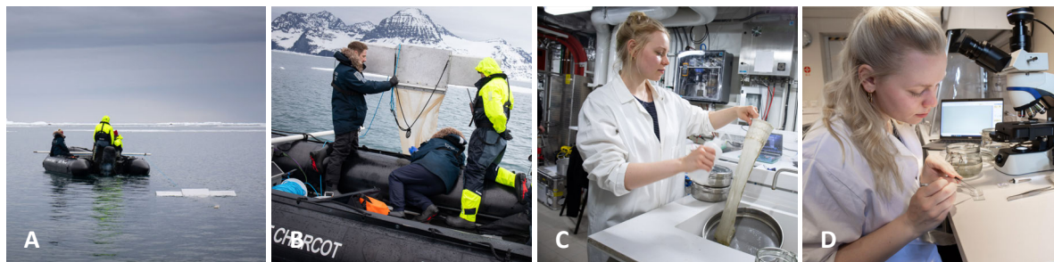
Fig. 13: Micro plastic sampling with the Manta Net (A and B) and processing of the sample material in the lab (C and D). Photo credit: Xavier Boymond.
