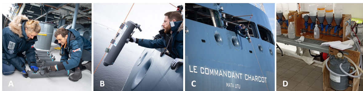
Fig. 7: Sampling of water masses from discrete depths from the afterdeck using Niskin bottles (A-C) for filtration in the lab (D) to determine phytoplankton pigments as well as particulate carbon and nitrogen concentrations. Photo credit: Xavier Boymond.
