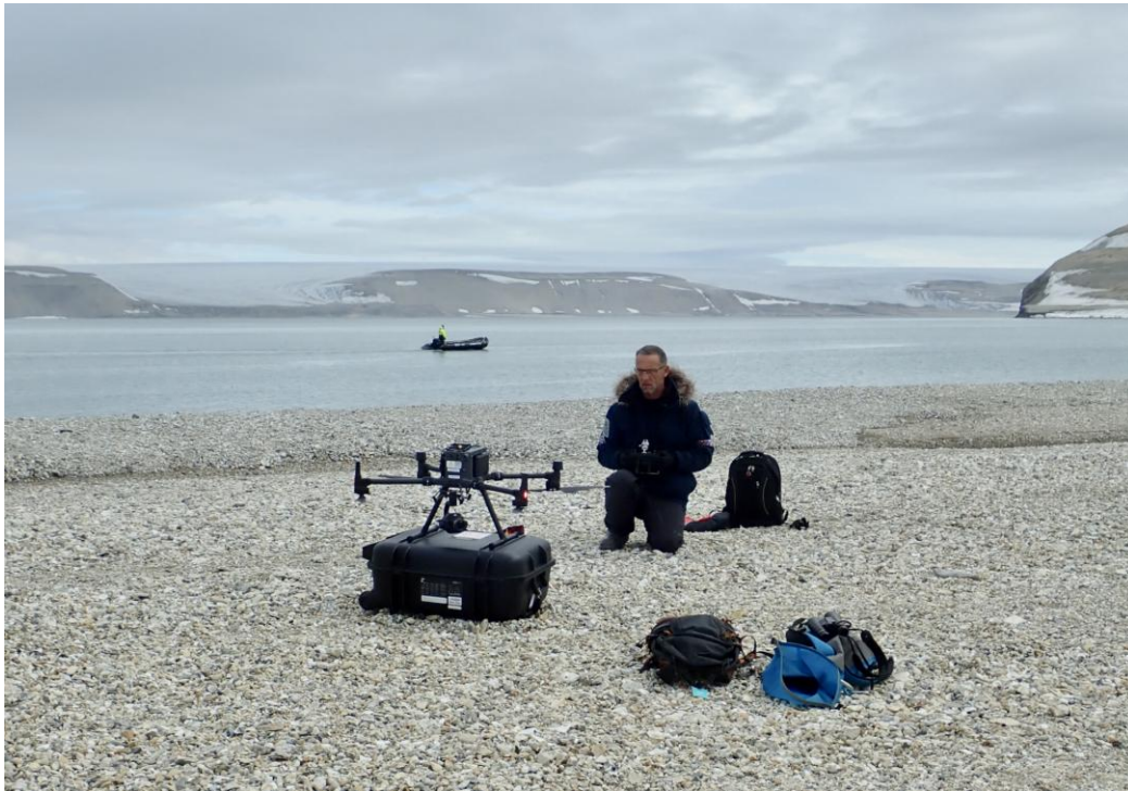
Figure 4.11: Measurements of a small glacier with the camera P1 from the beach
