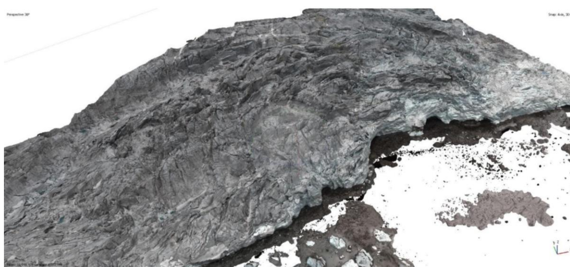
Figure 5.7: At the top, an overall photo of the glacier front, with a zoom on caves, and at the bottom, the 3D model produced by photogrammetry from the images acquired by the P1 camera.
