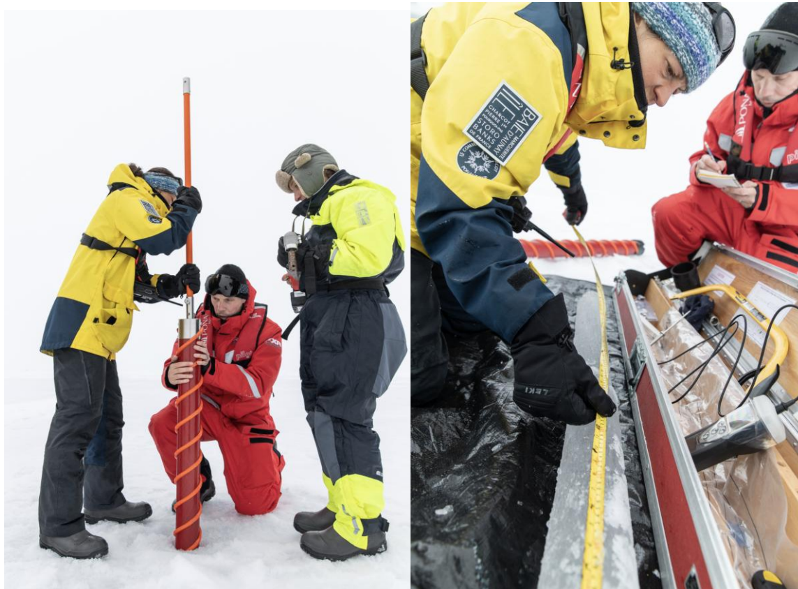
Figure 3.6: Ice coring and measurements of the main characteristics of the ice.
