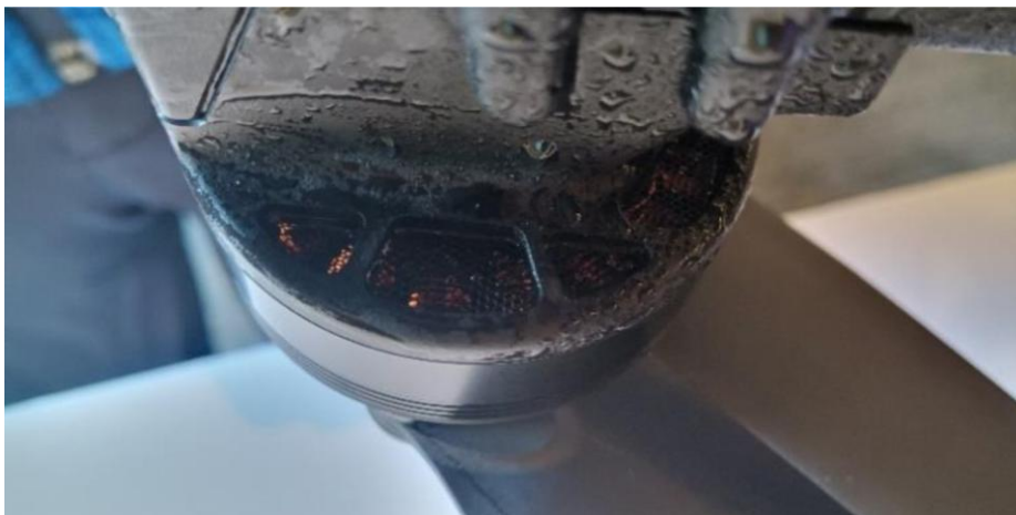
Figure 4.8: stators covered with melt ice
