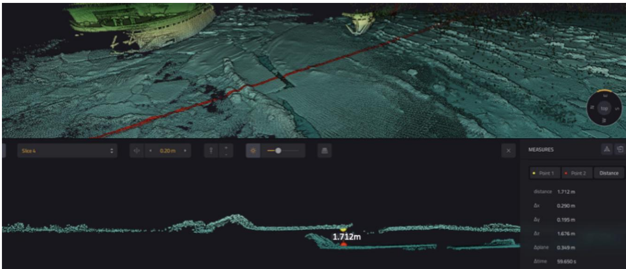
Figure 5.4: the bottom image corresponds to the red cut of the top image. We can observe an important height difference of 1.71m between two measurements of the same floe. This difference is due to the insufficient precision of the altitude of the drone. This problem could probably be solved using the PPP-AR GNSS post-processing.
