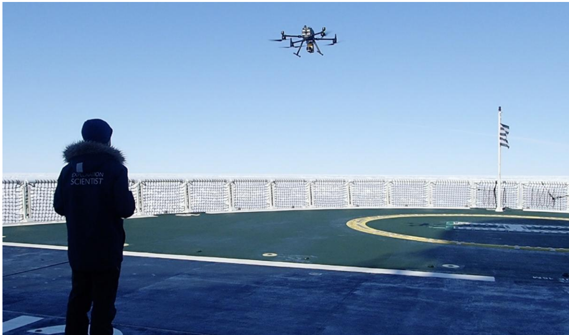
Figure 4.5: Take off from the helideck for sea ice measurements with the 3D lidar scanner.
