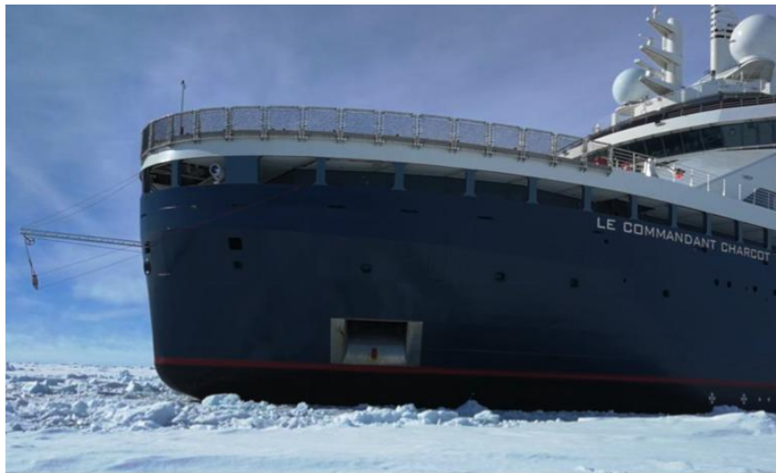
Figure 3.4: Sea Ice Measurement Sensor (SIMS) that is suspended at the front of the boat when it is in the ice pack to measure the thickness of the ice.
