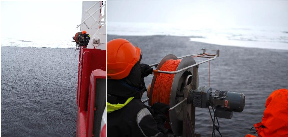
**Figure 2.18 - the line being payed out over the stern of the ship (left) and reeled in using the boom on the winch to guide the line onto the drum equally**
