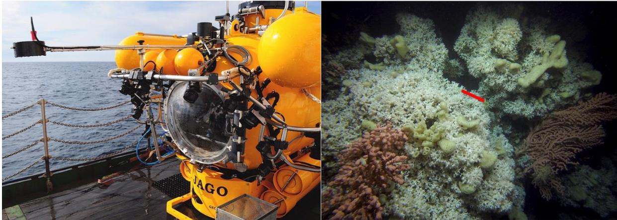
**Fig. 18:** Submersible JAGO on deck of RV POSEIDON with external GoPro-mini-camera in underwater housing mounted on an extension pole (left), right: one of the still images taken during one of the survey dives at Nord-Leksa. Red bar indicates the distance between the two laser points (20 cm). Pictures: JAGO-Team.
