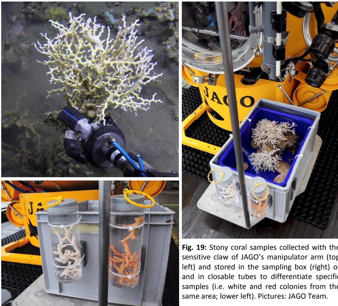
**Fig. 19:** Stony coral samples collected with the sensitive claw of JAGO's manipulator arm (top left) and stored in the sampling box (right) or and in closable tubes to differentiate specific samples (i.e. white and red colonies from the same area; lower left). Pictures: JAGO Team.
