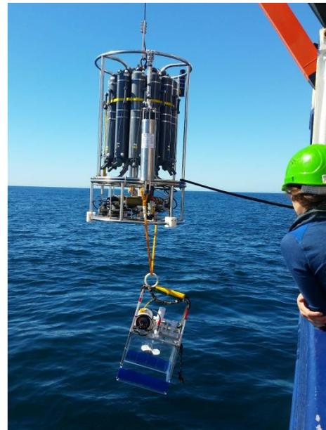
**Fig. 1:** Deployment of a CUBE with the CTD / water sampling instrument. (Picture: Janina Büscher)
