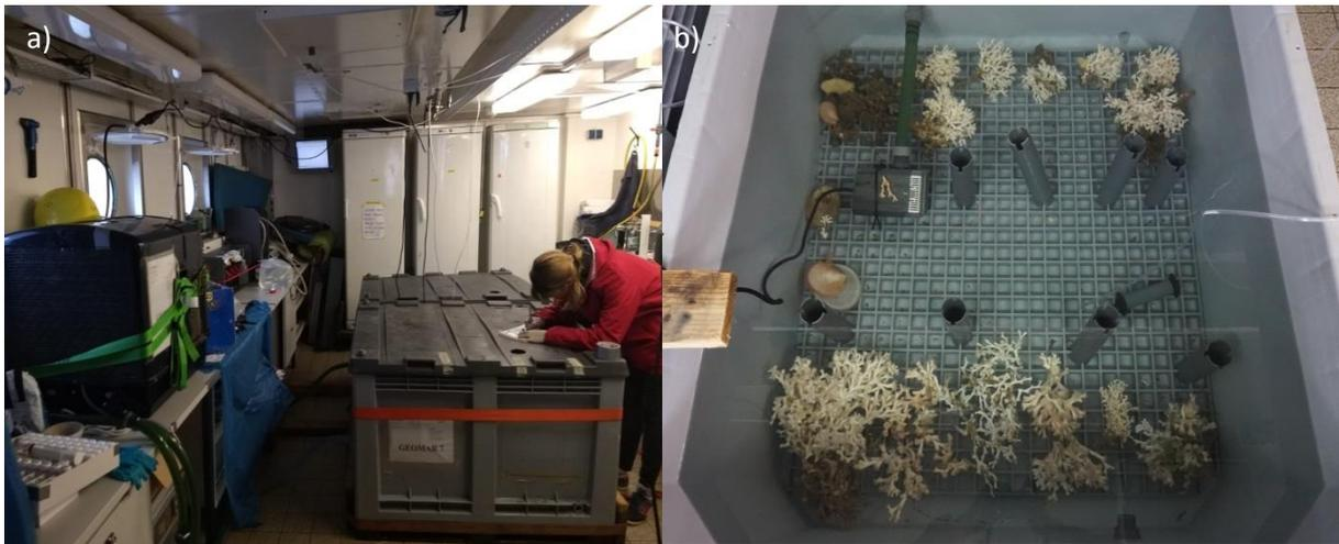
**Fig. 20:** Cultivation set-up with two large PVC tanks installed and secured in the middle of the wet lab of RV POSEIDON and connected to a cooler (left, picture a)). b) View into one of the cultivation tanks after coral collection, equipped with a grid and PVC spacers for purposes of assignment of coral groups. Pictures: a) Peter Striewski, b) Janina Büscher.
