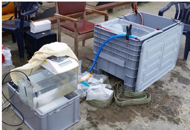
**Fig. 4:** Set-up of weighing facility on-shore in the port in Myre in front of the RV POSEIDON in order to weigh coral branches under water in a calm environment. Picture: Janina Büscher.
