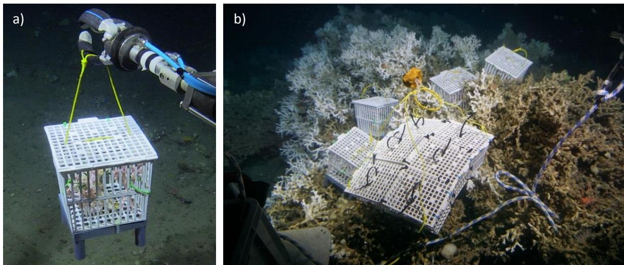
**Fig. 6:** *In situ* coral baskets with live labelled corals and a cluster of bioerosion baskets with dead coral fragments lifted with JAGO's manipulator arm (a) and deployed into the reef framework near living *Lophelia* colonies (b). Pictures: a) Karen Hissmann, b) Janina Büscher.
