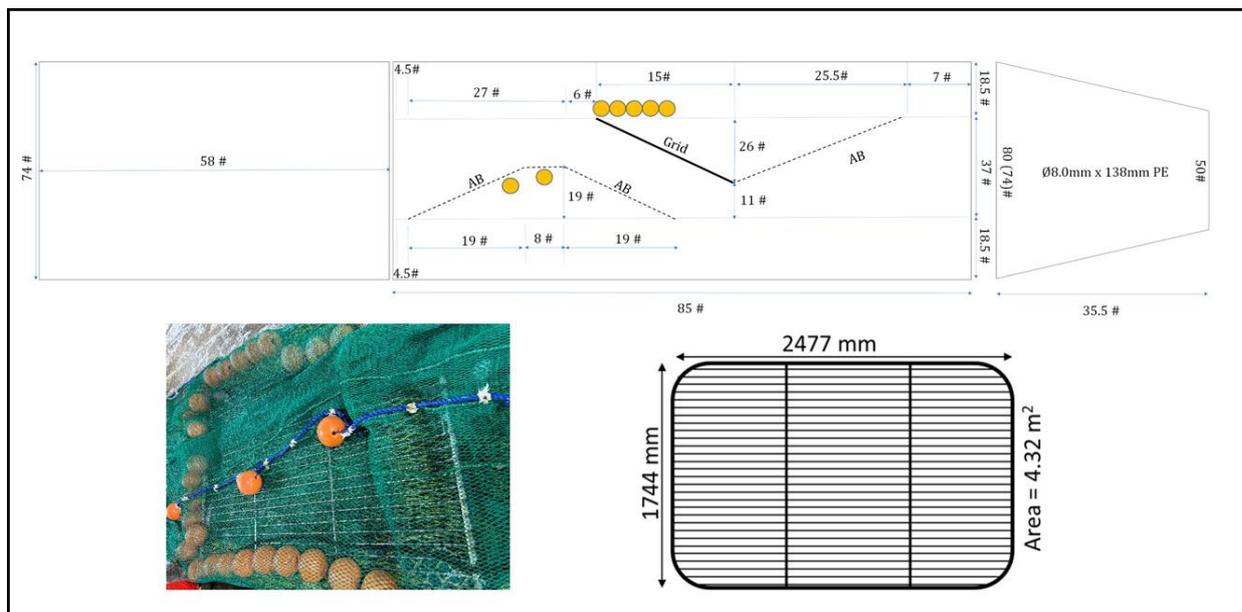
Figure 1. Illustration and schematics of the upscaled grid section.
