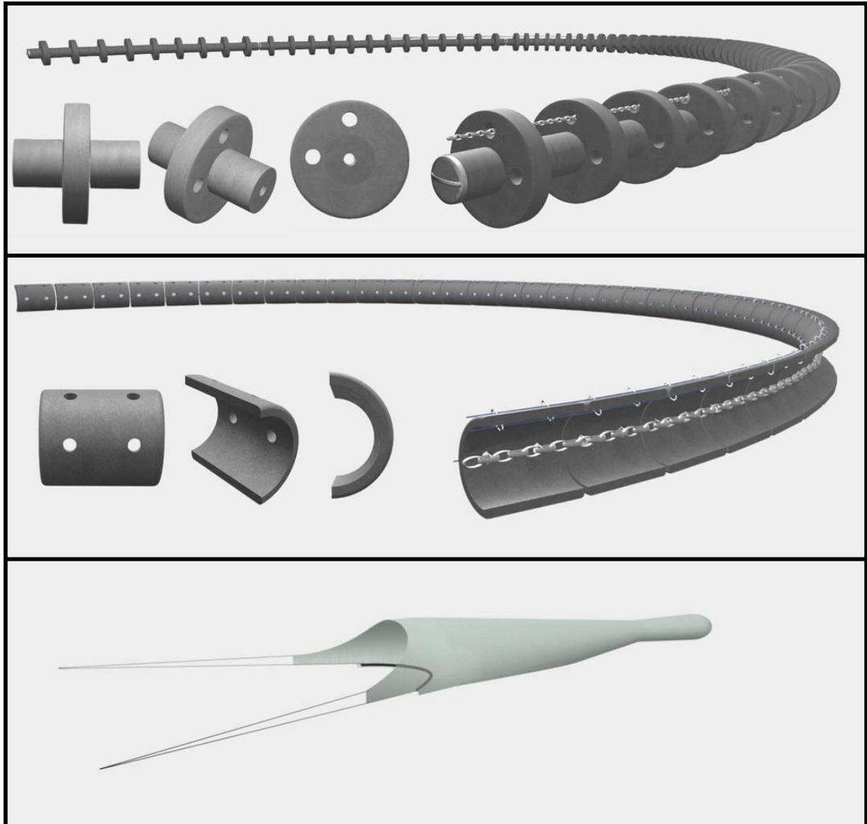
Figure 3. Schematics of the RH gear and the semicircular spreading gear.
