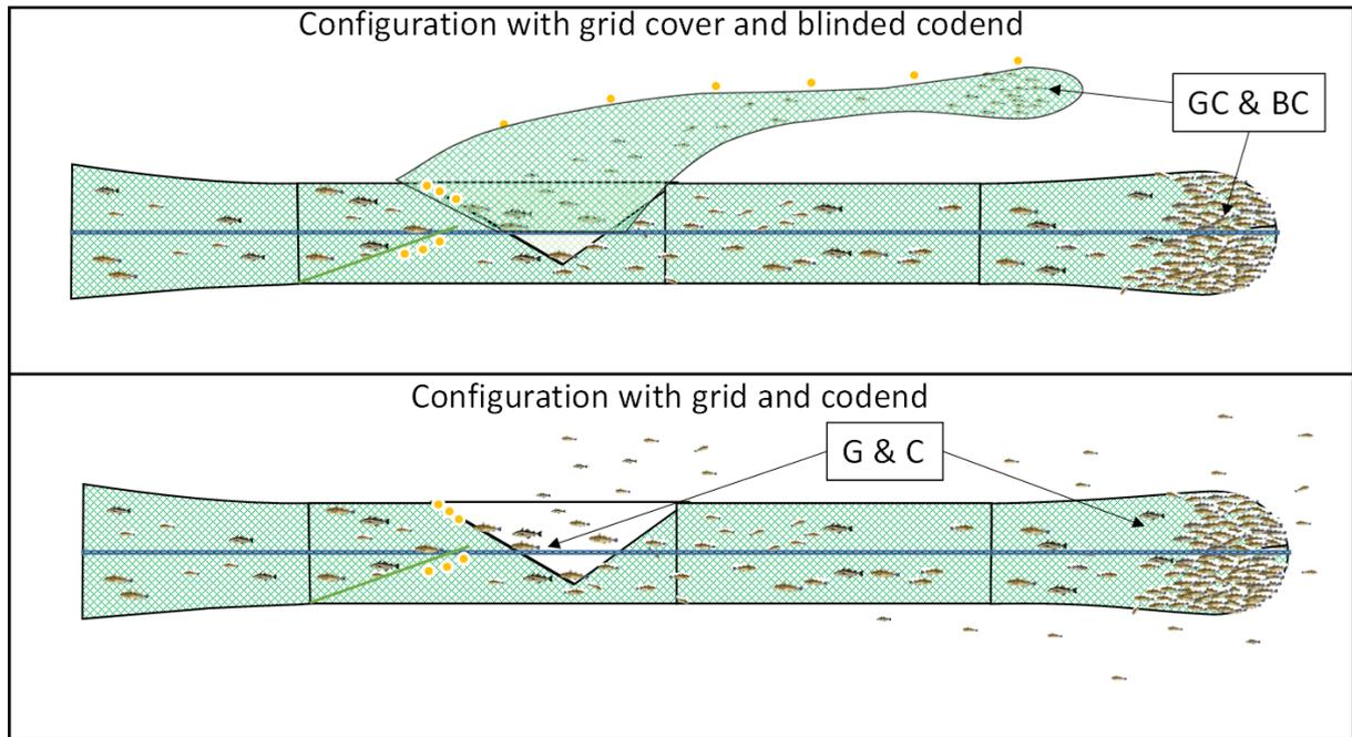
Figure 2. Schematics of the two configurations fished during the sea trials. Upper: Grid with grid cover followed by a blinded codend. Lower: Commercial configuration with uncovered grid and selective codend.
