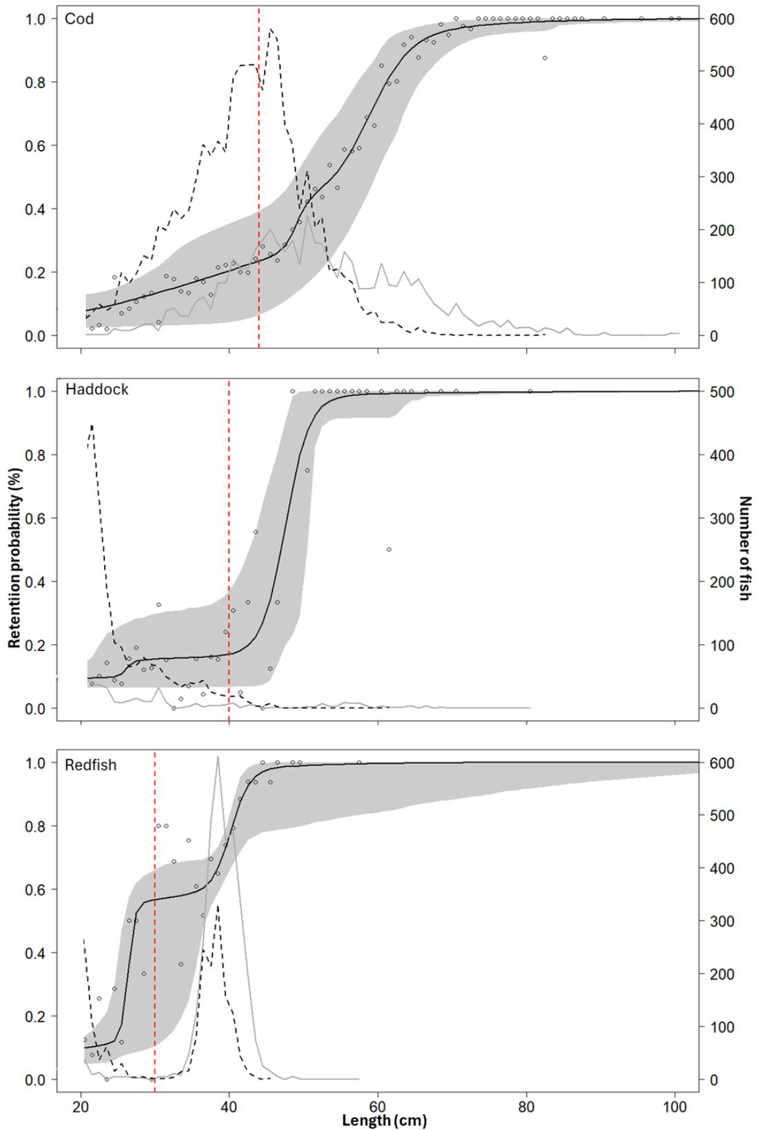
Figure 4. Size selectivity curves (black curve) for cod (upper), haddock (middle) and redfish (lower) with corresponding 95% confidence bands (gray area). The black circles denote the experimental data, the black stippled line the catch in the cover, the gray solid line the catch in the codend, and the vertical stippled line the MS for the respective species.
