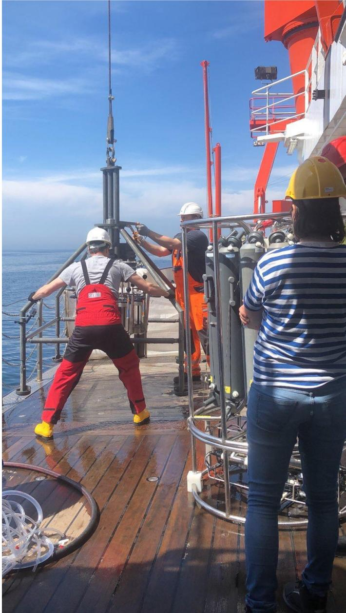
**Figure 9.1.2:** CTD measurements / deployment of CTD rosette [Photo: Chantal Mears / Hereon]
