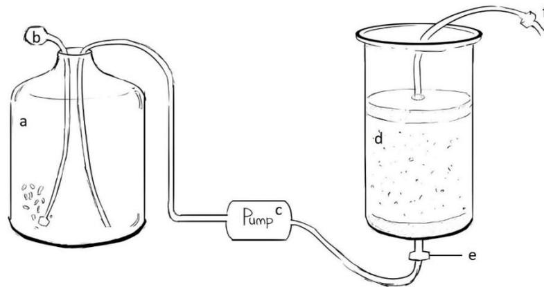
**Figure 5.3.4.1:** FTR incubation setup. a: water reservoir. b: aquarium pump aerating the FTR feedwater. c: peristaltic pump, pumping water from the reservoir through the FTRs. d: FTR containing homogenized sand. e: inlet sampling and flow through optode, measuring oxygen concentrations. f: outlet sampling and flow through optode, measuring oxygen concentrations.
