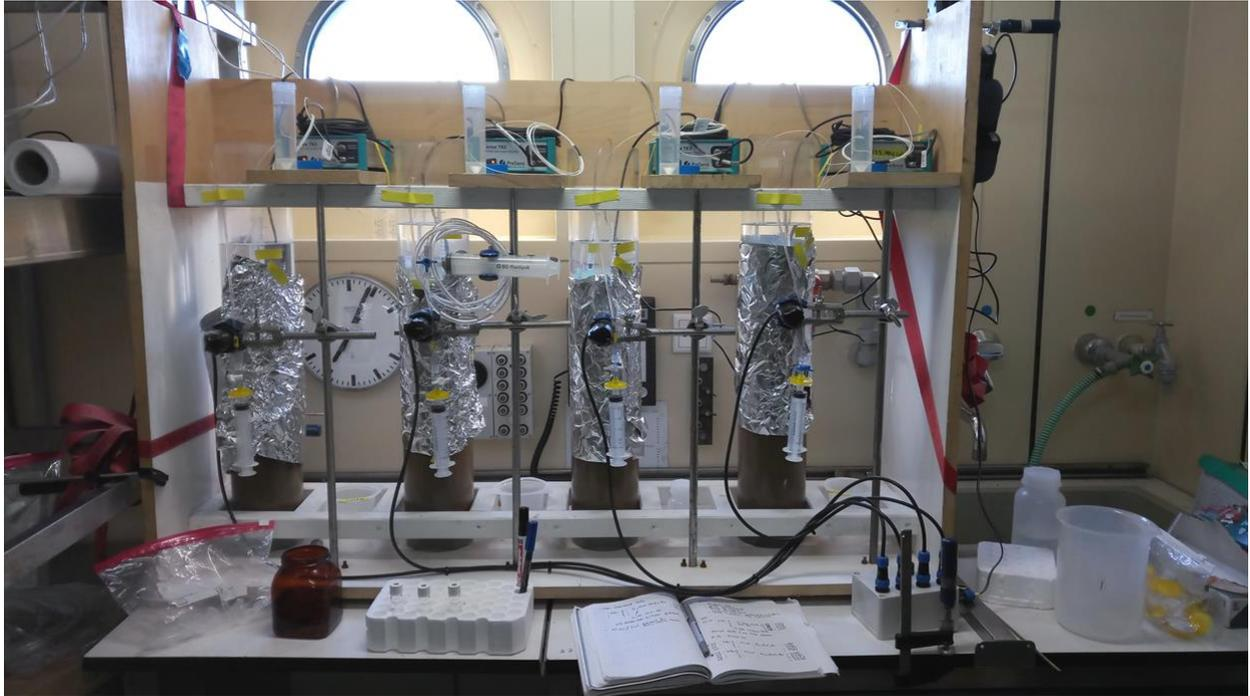
Figure 5.3.5.1: Photo of the whole-core incubation setup in the temperature-controlled lab of RV ALKOR. (Photo: C. Nantke)
