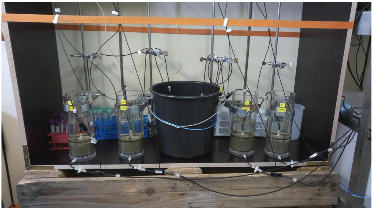
**Figure 5.3.4.2:** Photo of the FTR incubation setup in the temperature-controlled lab of RV ALKOR. (Photo: C. Nantke)
