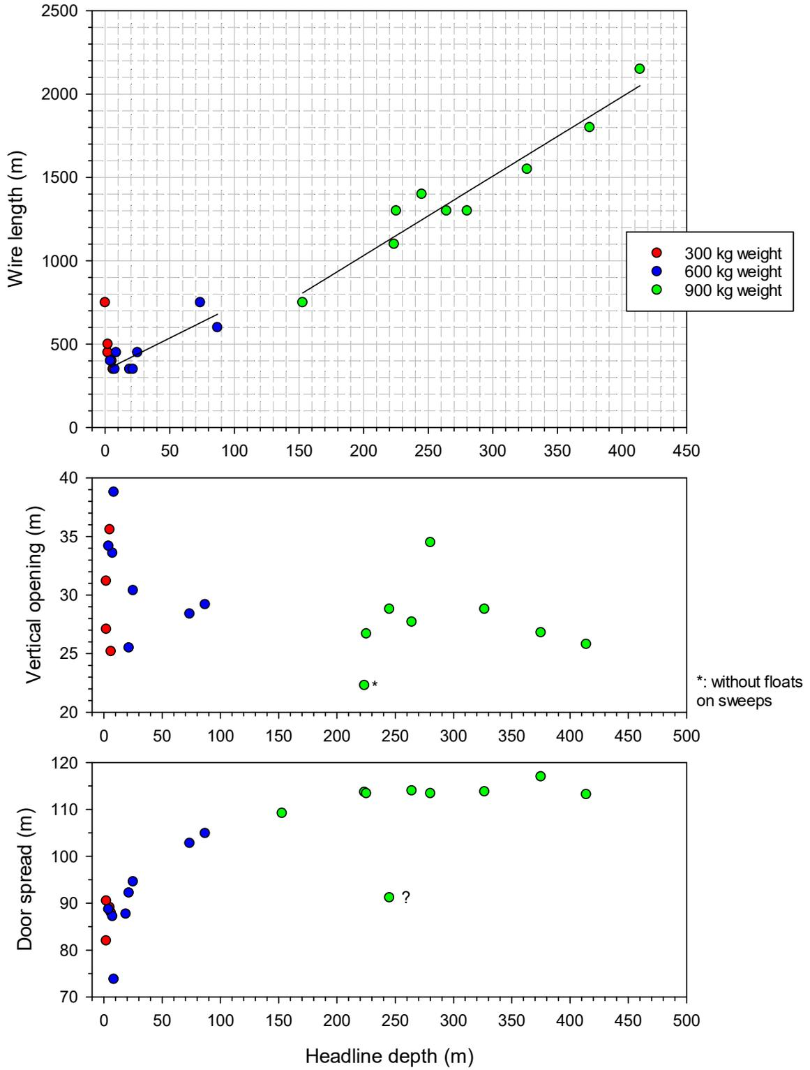
Note: Headline depth, door spread and vertical opening are average values from Scanmar plot files (may differ from the manual entries in SIS (Ship Information System))
