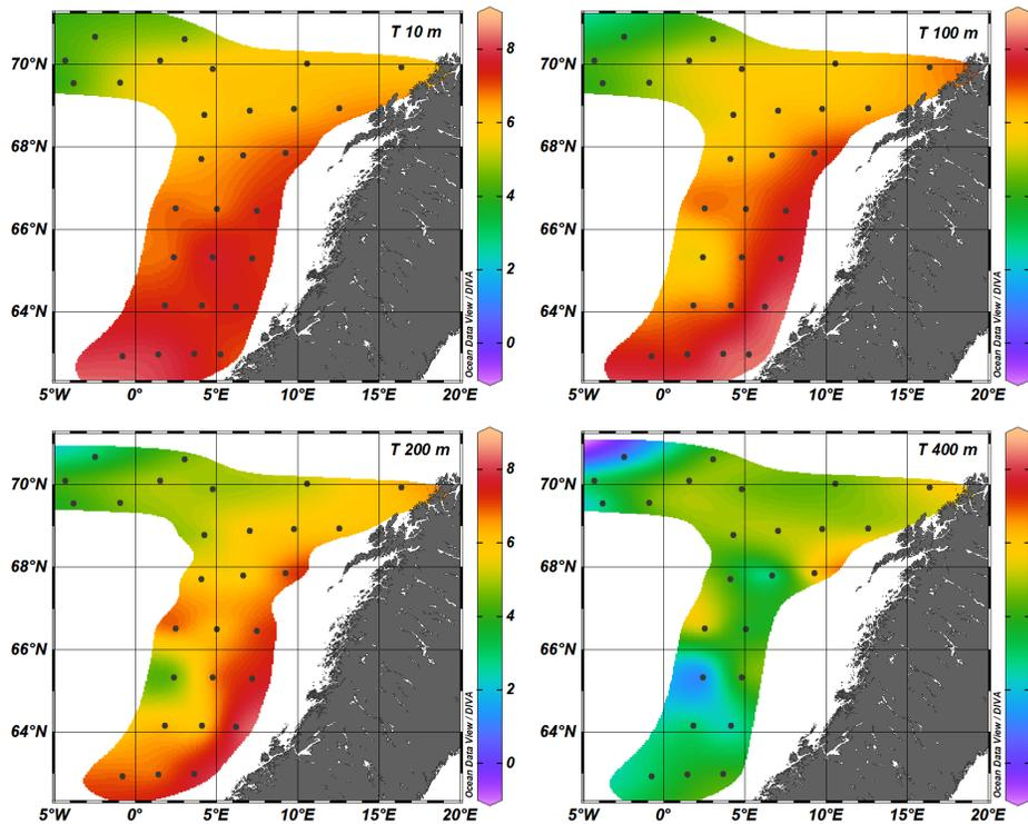
Figure 4: Horizontal temperature distribution in 10, 100, 200 and 400 m depth, R/V Dana IESNS 2020.
