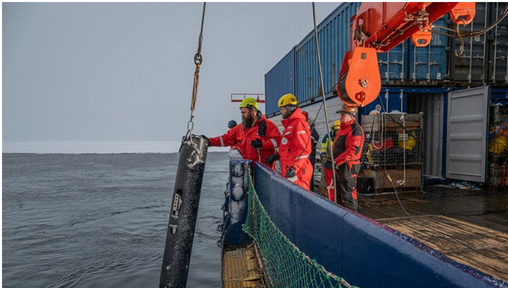
Fig. 1.5: The new pipe mooring for year-round hydrographic measurements. © Esther Horvath
