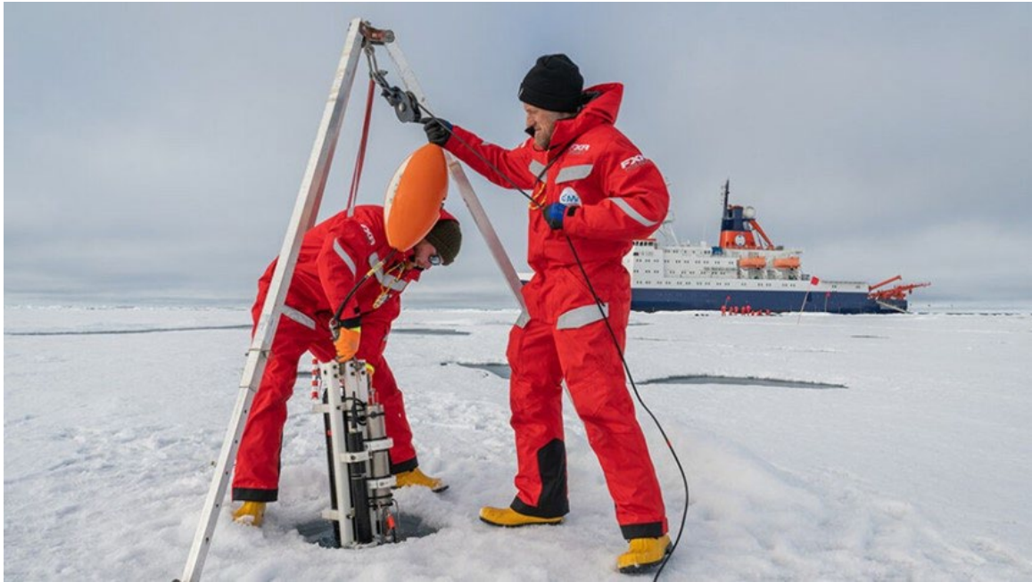
Fig. 1.4: Hydrographic work on the ice; here measurements with the "Suna" nitrate sensor, which measures nitrogen in water. © Esther Horvath
