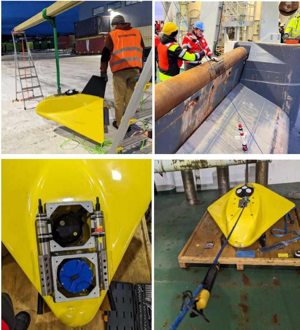
*Figure 6: Clockwise from top-left: Compass calibration on shore; deployment of concerto attached to the line via bale hose clamped to instrument+carabiner through loops on line; underside of V-Wing showing mounting of SBE37s and ADCP casings (downward facing instrument not included but case included for extra weight); attachment technique for solo Ts and Duets*
