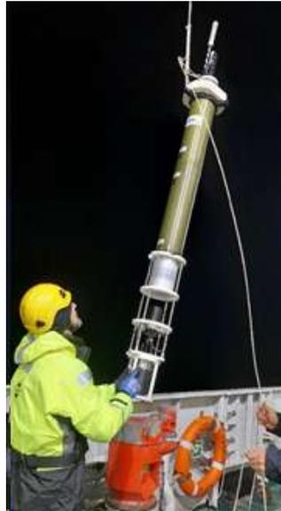
*Figure 15: The CMRE acoustic float being deployed with the crane off the starboard side .*
