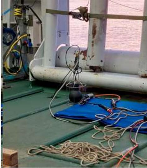
Figure 17: The Neptune D/11/BB source waiting to be lowered on the aft deck, starboard side, between periods of sound transmission.
