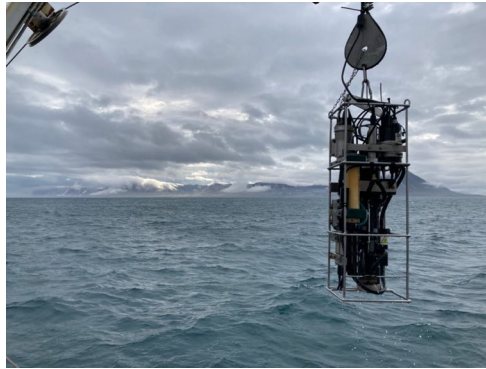
Figure 9. Optical-hydrological probe for measuring the inherent optical properties of sea water.
