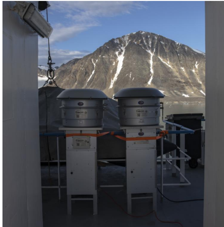
Figure 2. High volume air samplers installed onboard the expedition vessel.
