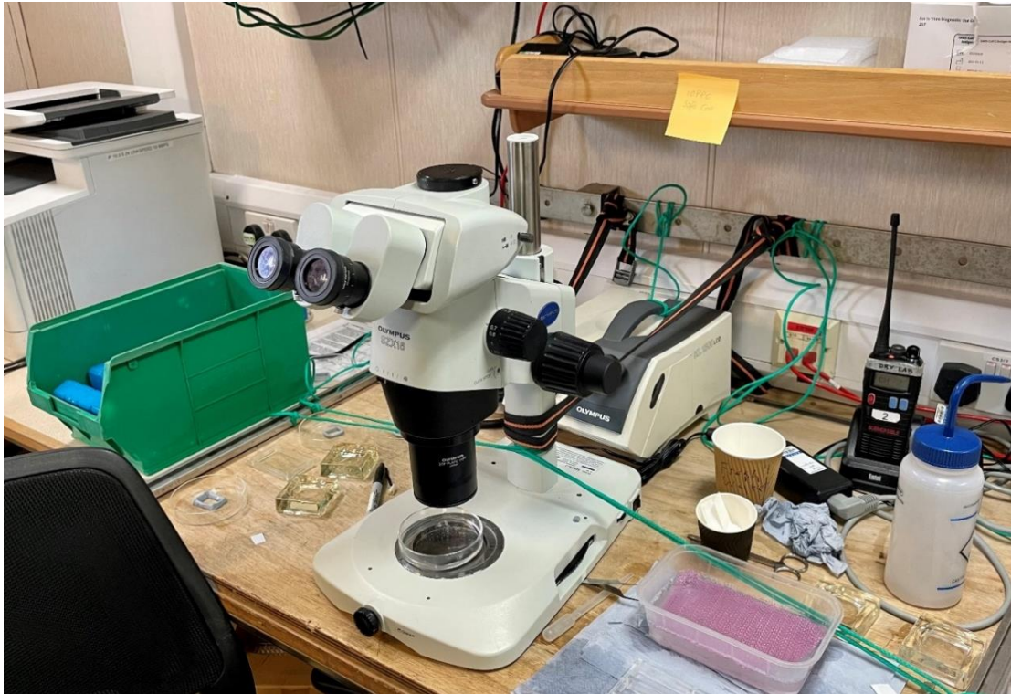
Figure 7. Stereo microscope and reflected top and bottom light used to identify and remove all ichthyoplankton eggs and larvae from samples.
