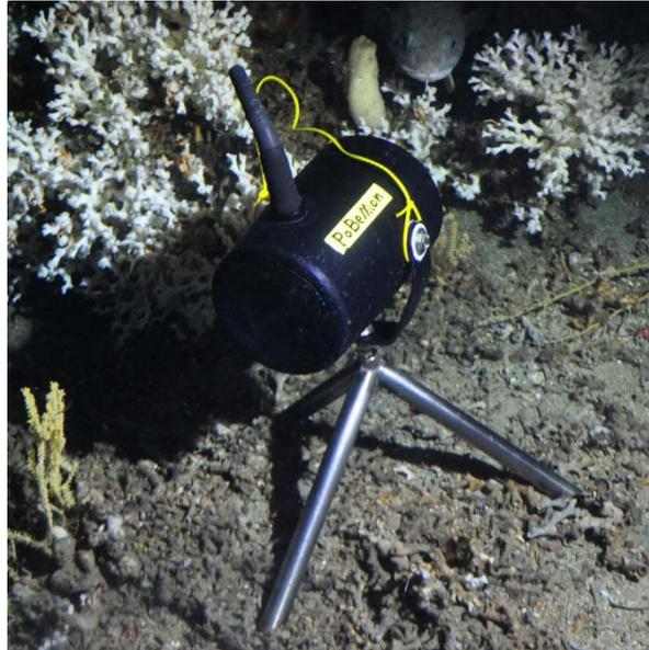
**Fig. 7** Underwater video camera placed in front of a single *L. pertusa* colony for natural polyp behaviour monitoring in the bottom region of the Nordleiksa Reef structures (Photo: JAGO team).
