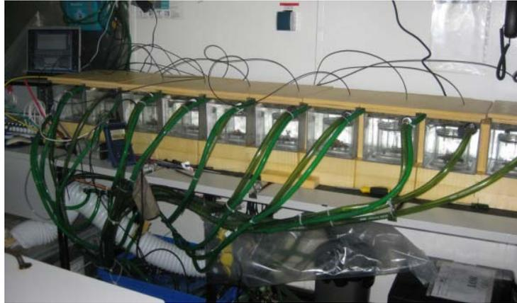
**Fig. 8** Experimental setup of short-term oxygen consumption measurements within closed respiration chambers in the wet laboratory of RV POSEIDON (Photo: Janina Büscher).
