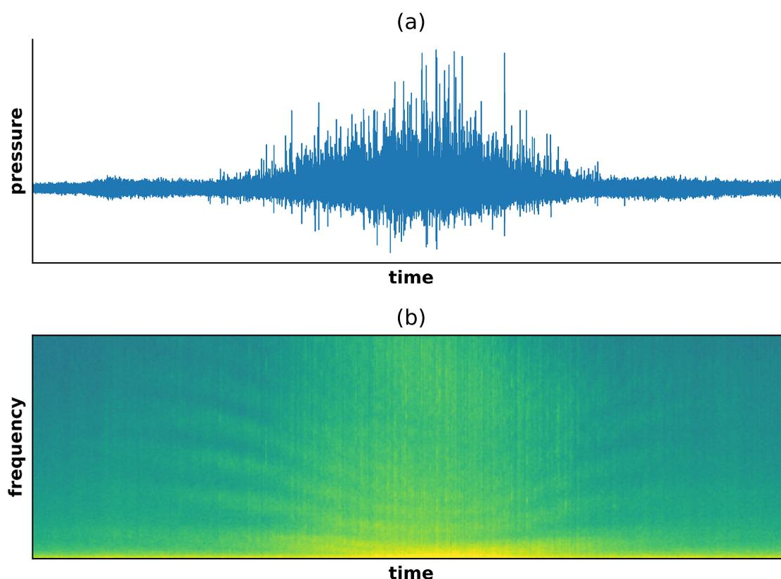
Figure 2: Measured signal (a) and resulting spectrogram (b) of a passing cargo vessel, with the closest point of approach (cpa) being approximately at the middle of the time axis.
