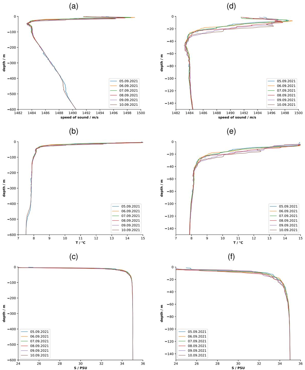
Figure 4: Vertical profiles of sound speed (a,d), temperature (b,e), and salinity (c,f) in central Sognefjord south of Høyanger. In the figures on the right (d,e,f) the upper 150 m of the respective deep profiles (a,b,c) are depicted.
