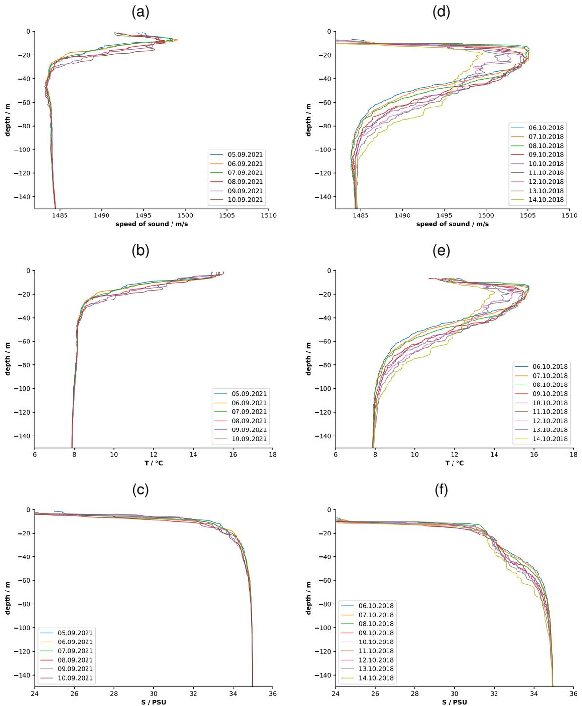
Figure 5: Comparison of the profiles of sound speed (a,d), temperature (b,e), and salinity (c,f) in central Sognefjord south of Høyanger. The figures on the left (a,b,c) correspond to the research cruise ARCAS2021, the figures on the right (d,e,f) to the previous research cruise ARCAS2018 [2].
