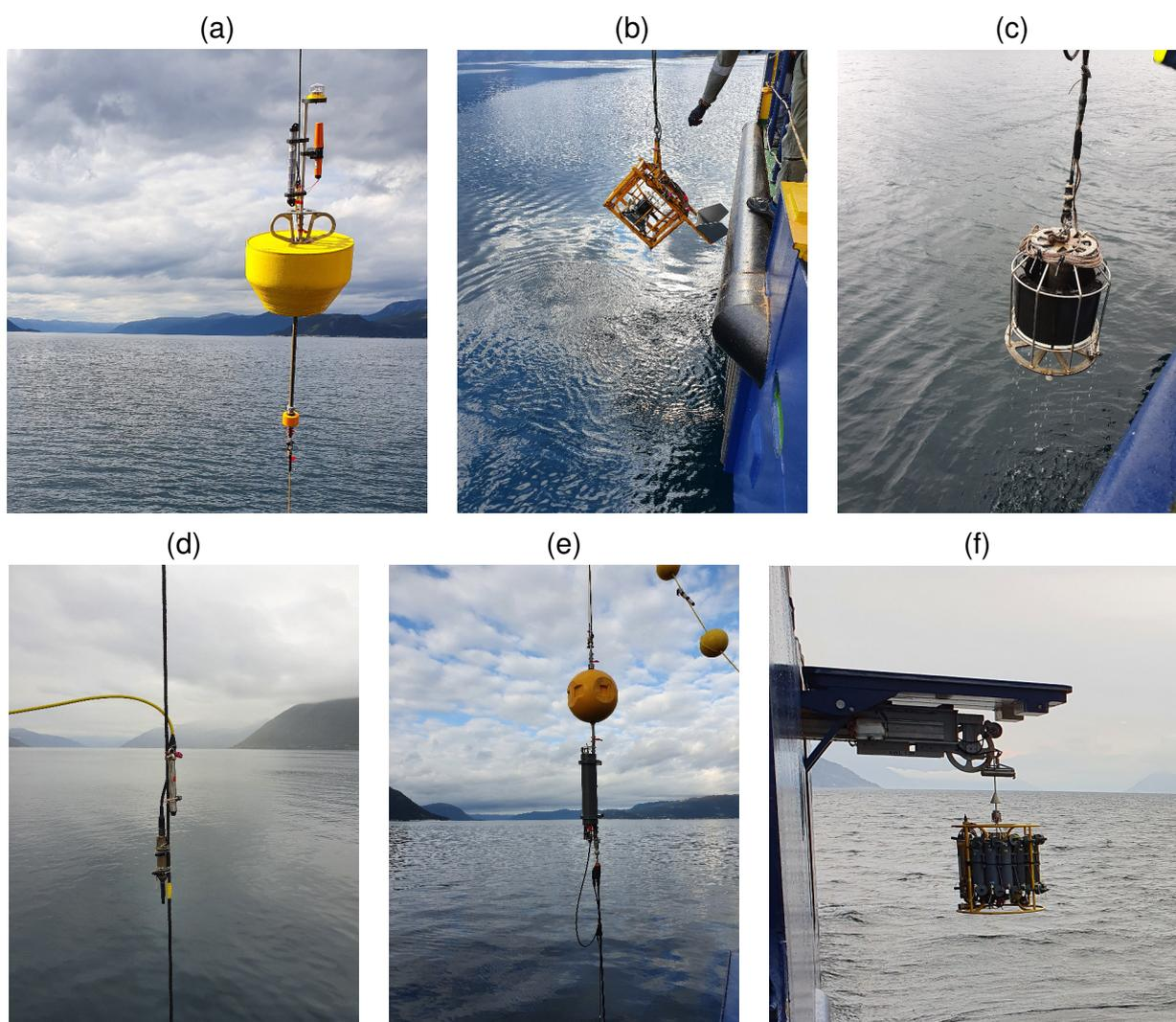
Figure 3: Pictures of measurement equipment used during ARCAS2021: communication unit of drift buoy (a), spherical transducer (b), flooded ring transducer (c), hydroacoustic receiver (d), hydroacoustic array (e), and CTD probe installed on-board of RV ELISABETH MANN BORGESE (f).
