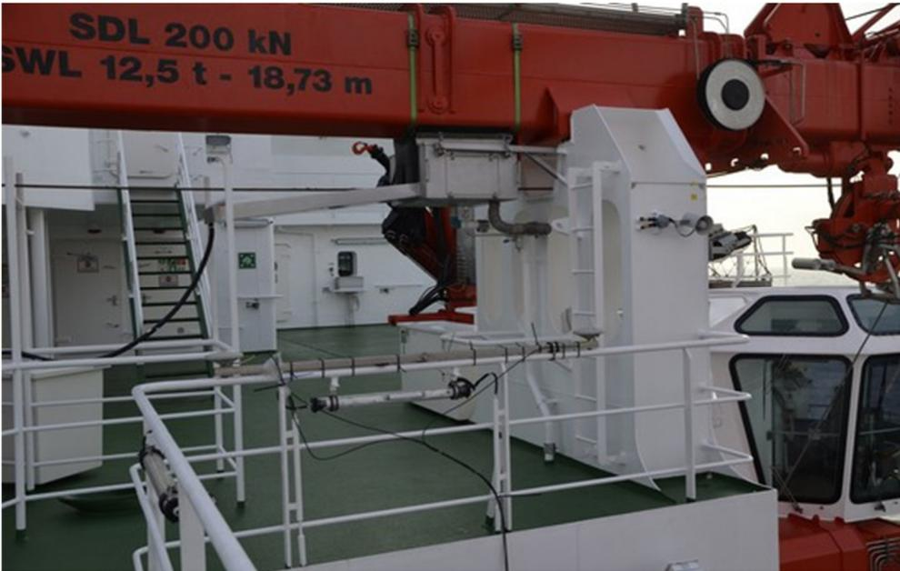
**Fig. 5.9** Installed antenna on the handrail, yellow deck.
