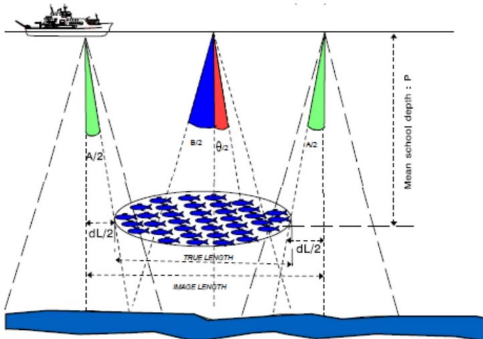
**Figure 1.** Schematic of a conical acoustic beam periodically sampling a relatively stationary fish school located between a hull-mounted transducer and the seabed as a ship moves from left to right (from Diner, 2001). The nominal beamwidth ( $\theta$ ) is the angle between half-power points (one-way) relative to the beam axis.
