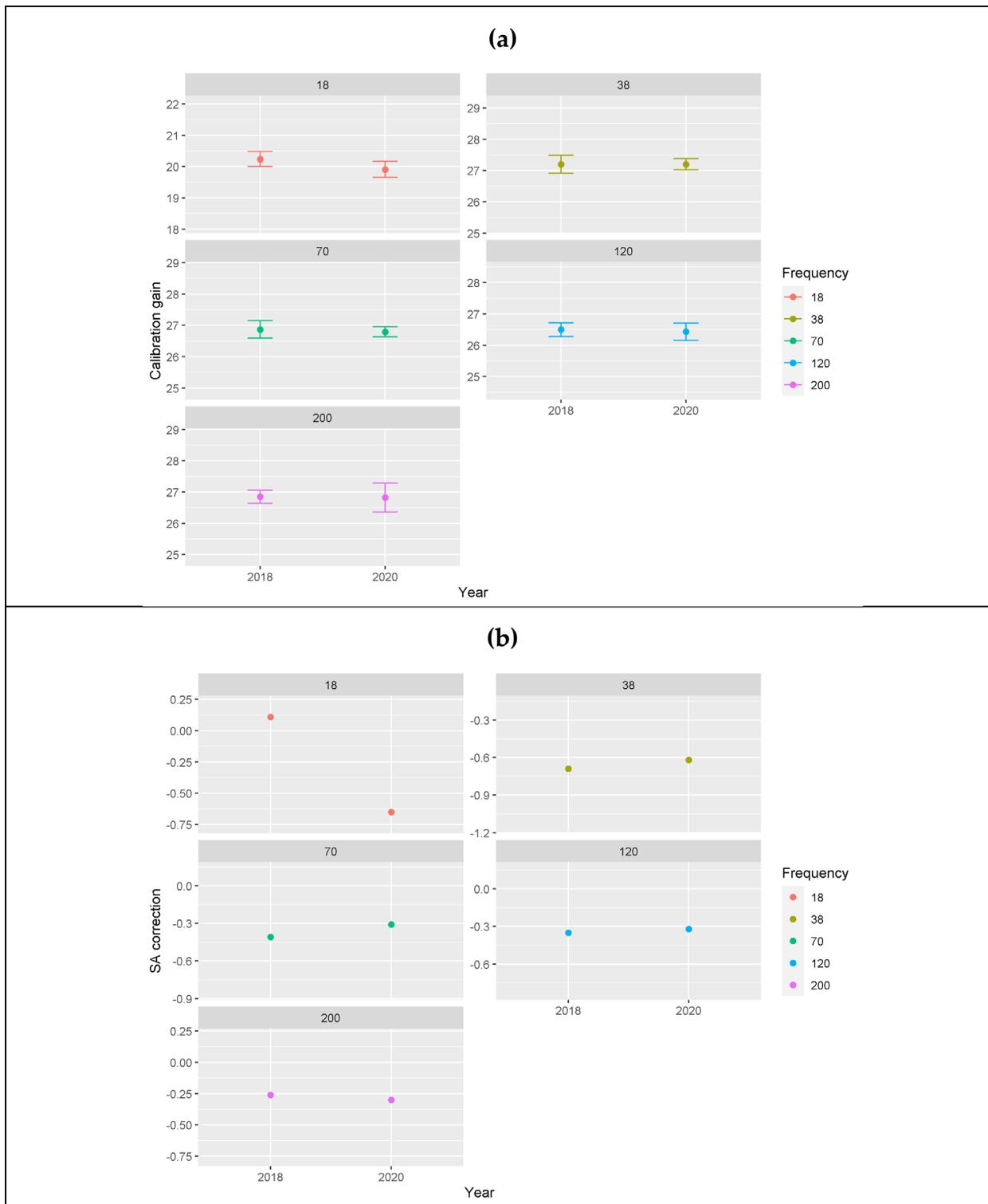
**Figure 2.10.** Calibration results from the Alida FV. Results of the 2020 survey are compared to those from the 2018 6aN survey. (a) Calibration gain with error bars reflecting RMS error for each measurement. (b) Sa correction.
