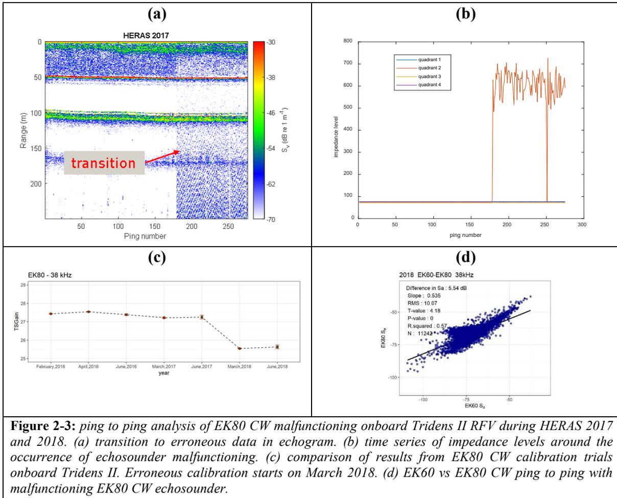
**Figure 2-3:** ping to ping analysis of EK80 CW malfunctioning onboard Tridens II RFV during HERAS 2017 and 2018. (a) transition to erroneous data in echogram. (b) time series of impedance levels around the occurrence of echosounder malfunctioning. (c) comparison of results from EK80 CW calibration trials onboard Tridens II. Erroneous calibration starts on March 2018. (d) EK60 vs EK80 CW ping to ping with malfunctioning EK80 CW echosounder.
