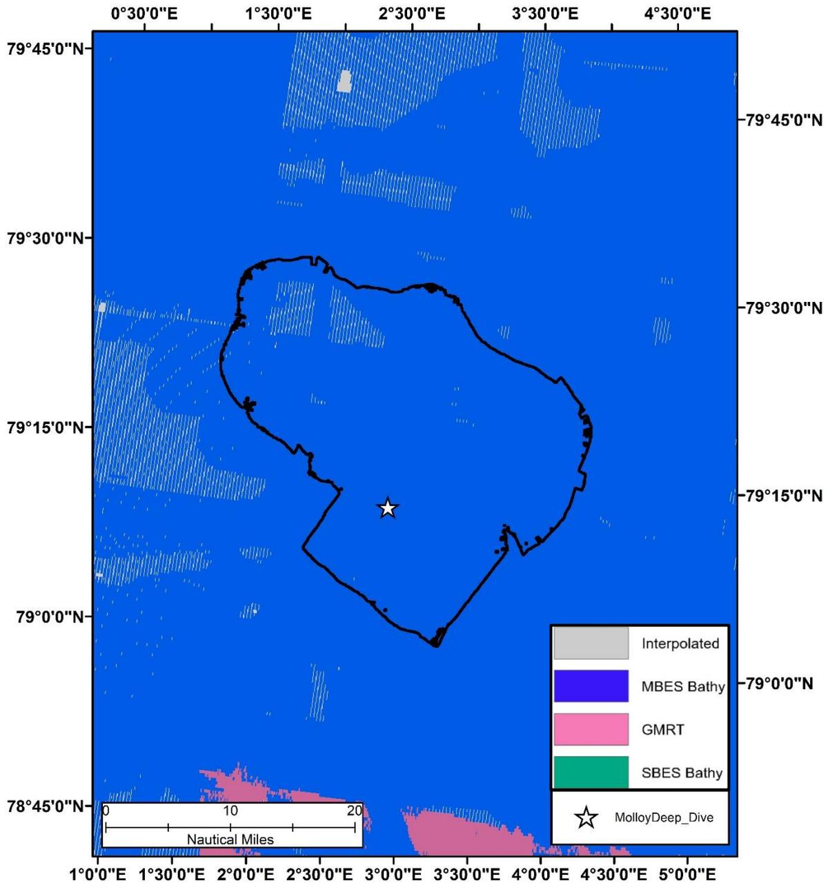
Figure 7: GEBCO data sources. Grey represents areas that were interpolated, and blue and pink are previously collected bathymetry data. The black outline is the area in Molloy where EM 124 data were collected.
