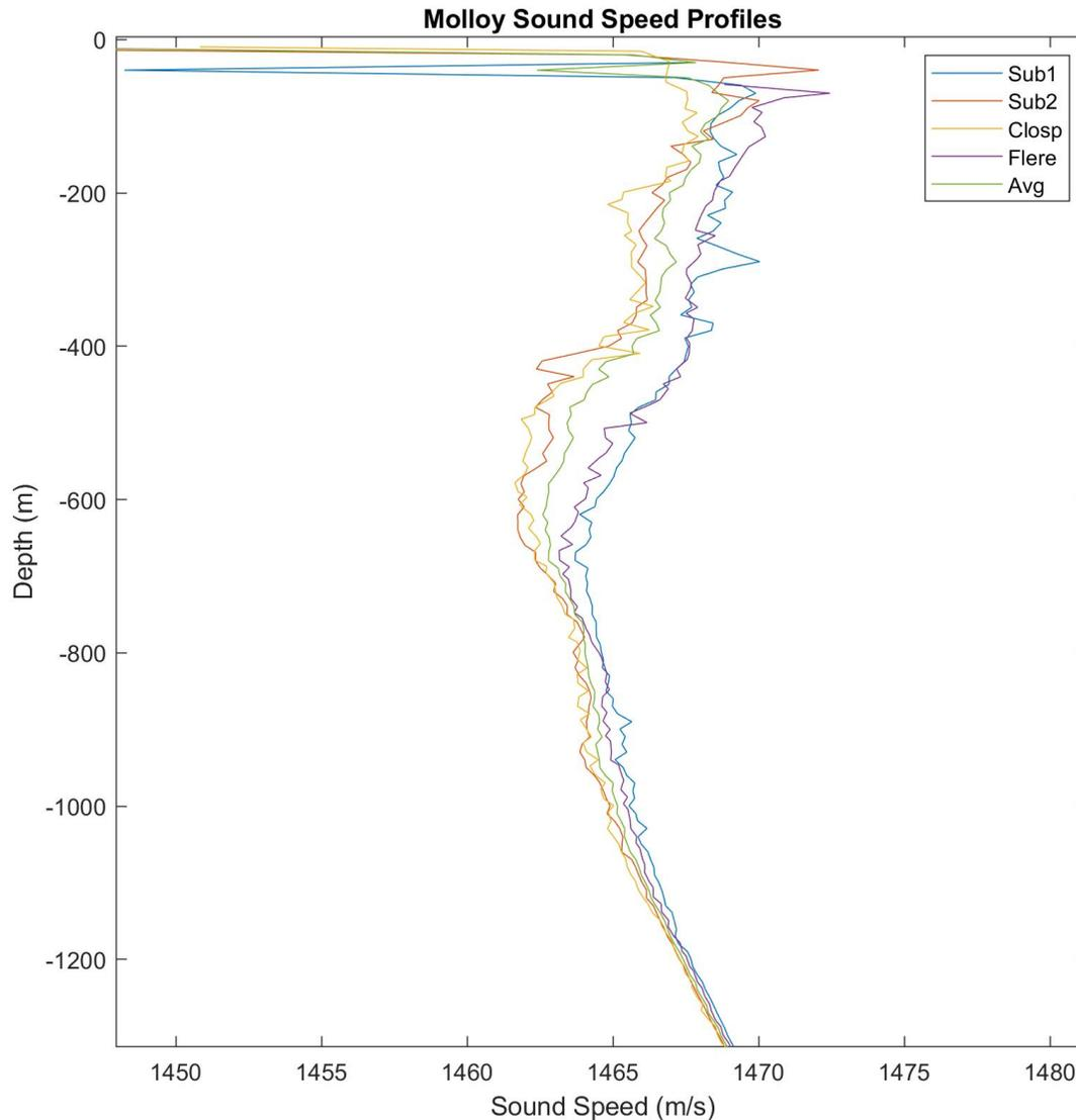
Figure 8: Sound Speed Manager comparison of all collected sound speed profiles from sub and XBT.
