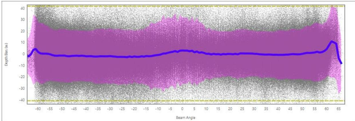
Figure 5: Molloy data (purple) in comparison with the IHO Order 1 specifications (yellow dotted lines). This figure proves these data meet the limitations set forth by the Order 1 survey classification.
