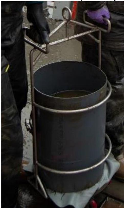
Figure 6.1b2 Transport of a core using the carrying frame and rolling platform across the deck
