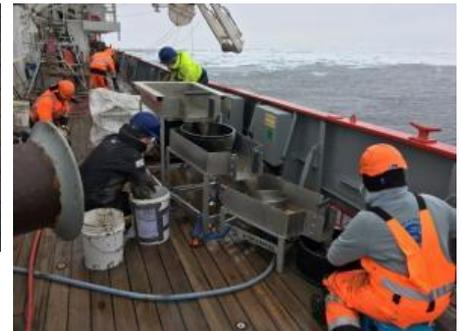
Figure 7.2c2 Image showing the sieve table set-up and the staged sieves.
