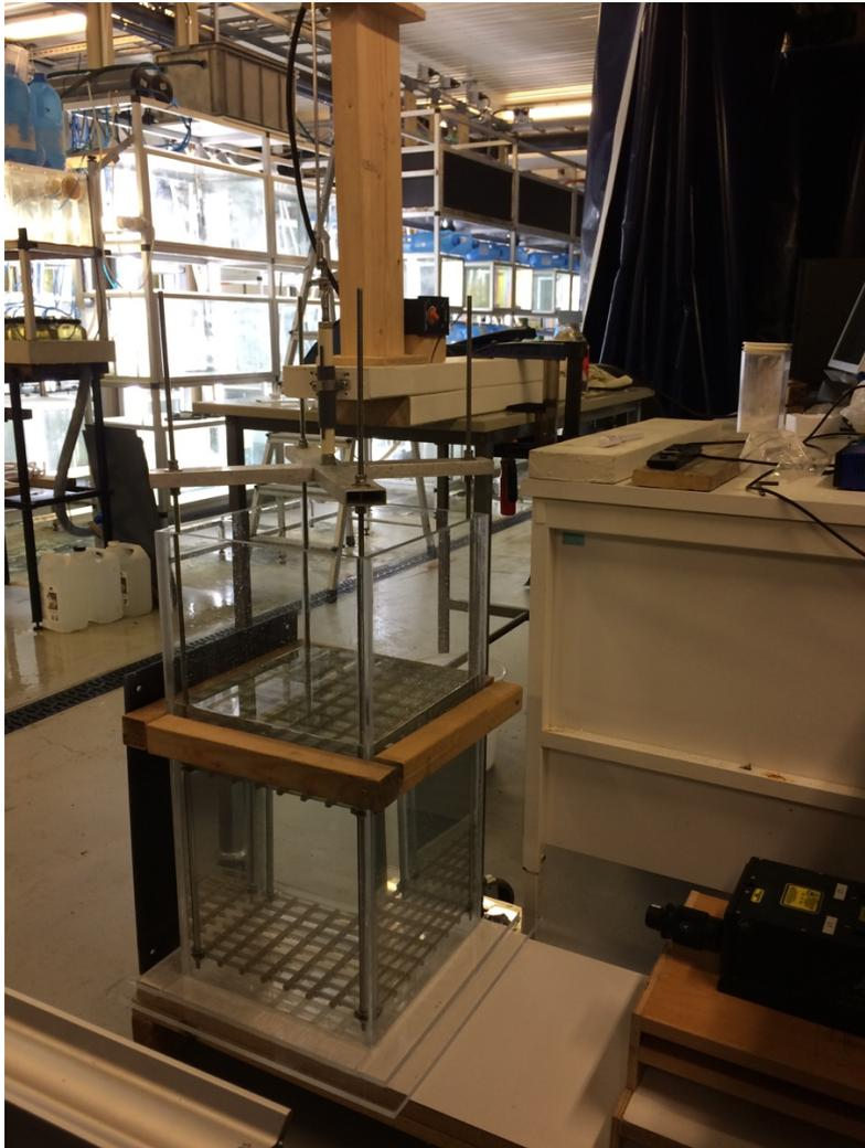
*Figure 3. Test setup of turbulence tank, camera and laser for simultaneous recordings of larval swimming and flow velocity vectors using Particle Image Velocimetry. Image courtesy of A. Larsson.*
