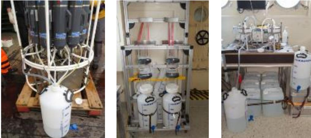
Figure 7 Seawater sampling devices used for size fractionation during the cruise.
