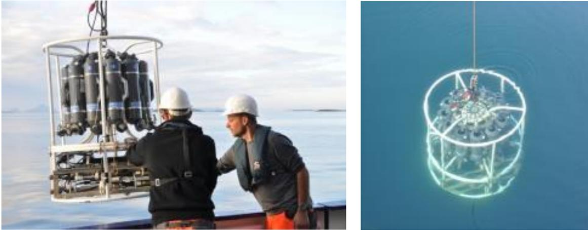
Figure 1 Onboard device Seabird 'sbe911+' CTD probe with sampling rosette for station work on R/V Heincke.
