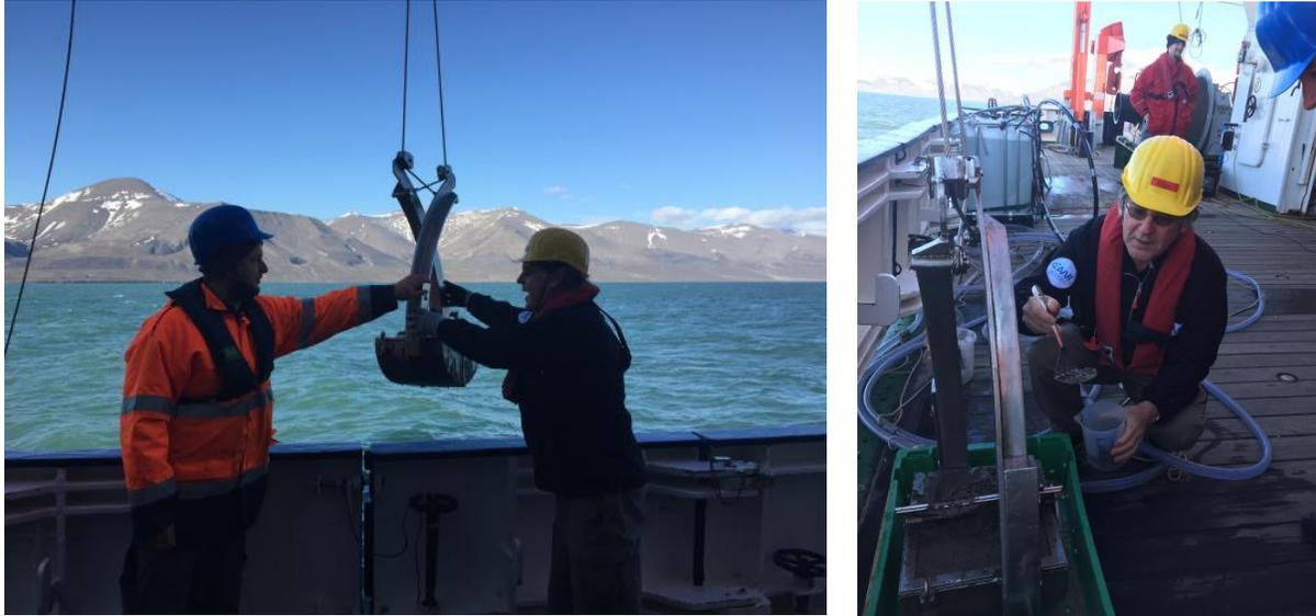
Figure 12 Benthic sediment samples collected with a Van Veen-type sediment grab sampler; left side grabber hived on board and right side detailed sampling of the sediment.
