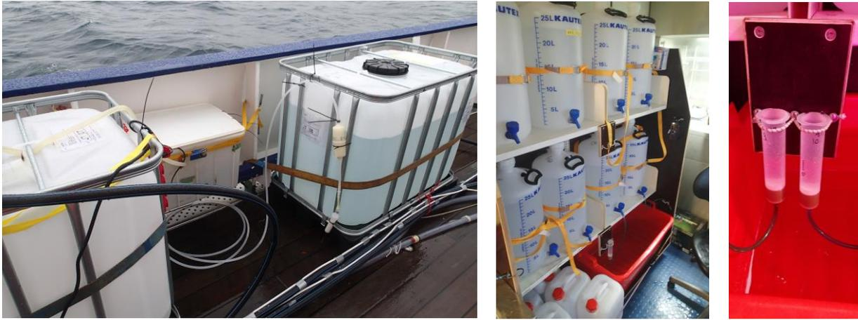
Figure 2 Large-scale DOM-SPM tank, filter and solid phase extraction for 600 L, 20 L and 0.5 L DOM concentration
