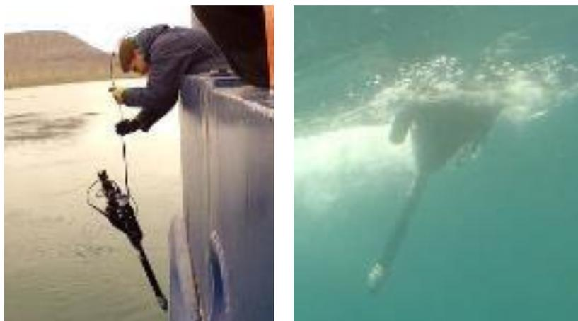
Figure 3 Hyperspectral profiling system Satlantic Inc. (Canada) to acquire bio-optical data during free fall mode from *R/V Heincke*.
