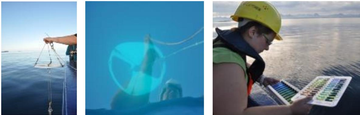
Figure 4 Secchi disc above and in water (left, middle) and Forel-Ule (FU) color comparator scale to determine the water color (right).
