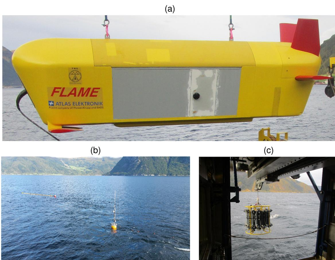
Figure 2: Pictures of measurement equipment used during *blueFLAME2017*: FLAME towed body measurement system during launching in Høyanger fjord (a), freely drifting projector buoy directly before recovering in Sognefjord (b), and CTD probe installed on-board of RV ELISABETH MANN BORGESE (c).
