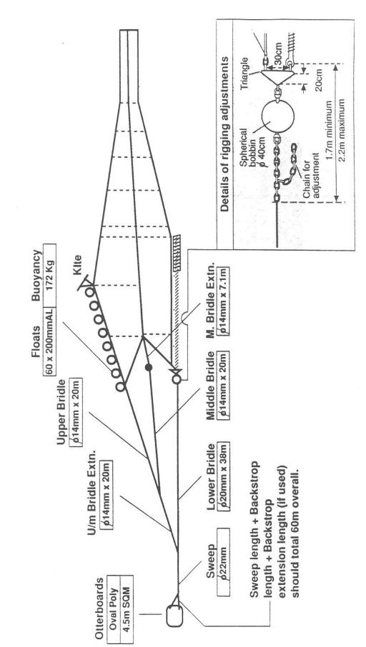
GOV 36/47 GROUND FISH SURVEY TRAWL : Overall rigging diagram
