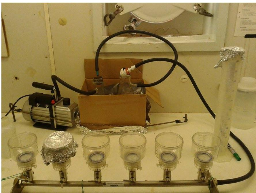
Figure 3: Filtration rig in R/V Skagerak lab.
