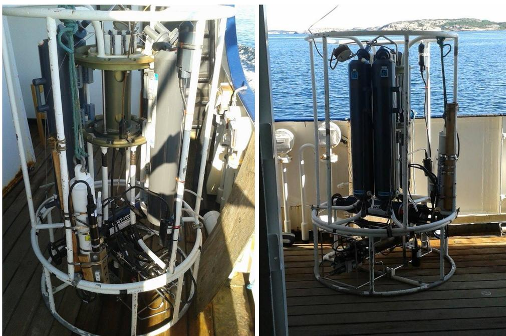
Figure 2: Rosette frame with main CTD (olive green, mounted horizontally lowest in the frame), auxiliary CTD (white plastic, mounted vertically), Niskin bottles (gray plastic, mounted vertically), LISST (black cylinder, mounted horizontally above main CTD).
