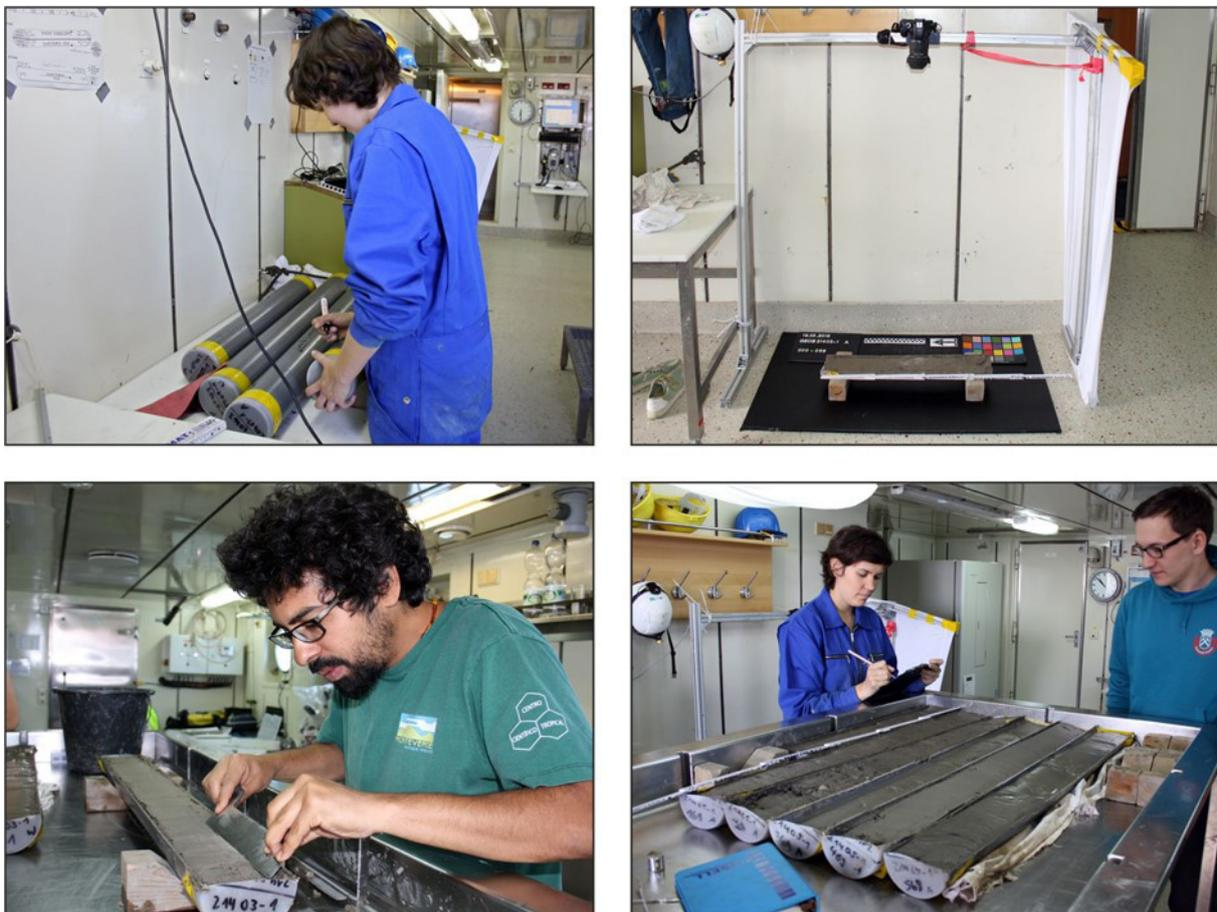
Fig. 5.9 Core handling and visual core description performed in the wet lab of RV Heincke. From left to right and up to down: core labelling, core imaging, core preparation for description, and core description
