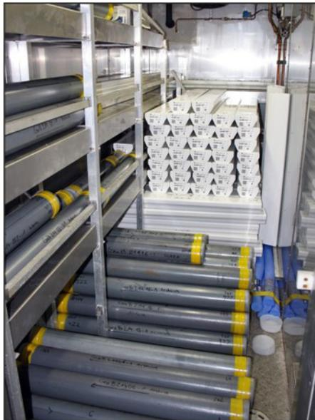
Fig. 5.8 Core sections stored at about 4°C in the reefer as whole rounds and half sections (D-tubes).
