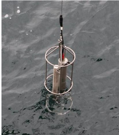
Fig. 5 CTD probe OTS 43 during deployment procedure.
