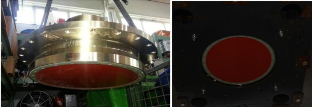
Fig. 3 ADCP RDI Ocean Surveyor 75 kHz before integration (left) and during integration (right) onboard EMB
