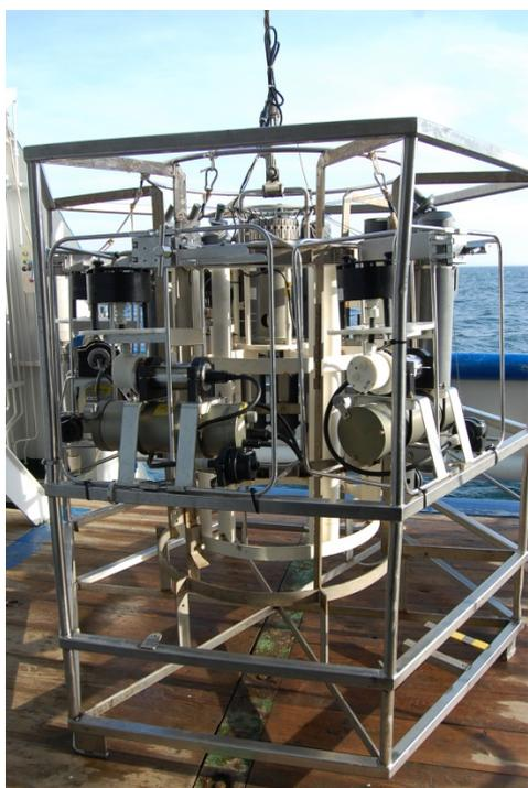
*Figure 1, Pumps mounted on the CTD frame*
