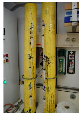
*Pore water sampling of piston core sections using rhizons*
