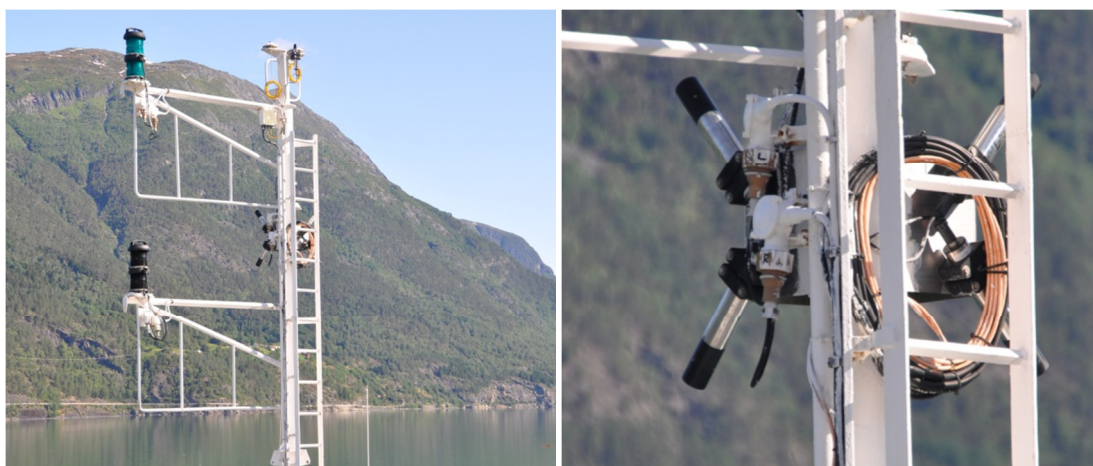
Figure 7 The radiometric setup on the foremast of R/V Heincke . One RAMSES-ACC hyperspectral cosine irradiance meter was installed at the top of the mast to measure total downwelling solar irradiance (yellow cable).
