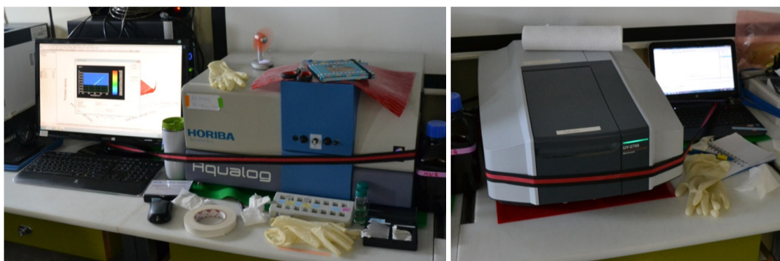
Figure 2 Aqualog® spectrofluorometer to determine absorbance spectra and fluorescence excitation-emission matrices (EEM) for CDOM/FDOM (left). Shimadzu UV2700 to determine CDOM absorbance spectra (right).
