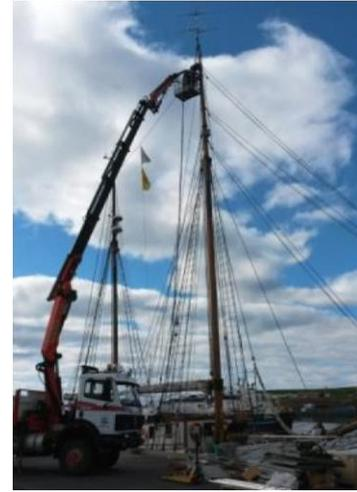
Figure 2. Left: Sailing vessel *Donna Wood* at sea. Note the long bow-sprit from which tags were attached using a hand-pole. Right: using a crane to mount VHF antennas on top of the 25m high foremast. Two downward looking video cameras were also placed near the antennae.
