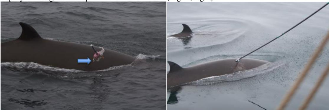
Figure 3. Left: Tagging attempt of a Dtag 2 on a Northern bottlenose whale using the ARTS launching system. The blue arrow points to the customized biopsy collection system attached to the ARTS carrier. Right: Tagging attempt of a Dtag 3 on a Northern bottlenose whale using the tag pole from the bowsprit.
