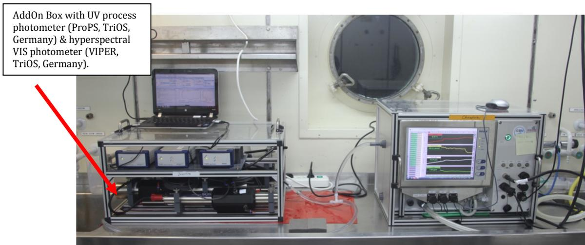
**Figure 4** PocketFerryBox (right) with AddOn box equipped with UV-/VIS spectrometers (left).
