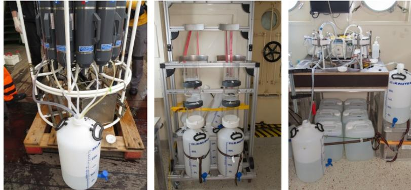
**Figure 8** Seawater sampling devices used for size fractionation during the cruise
