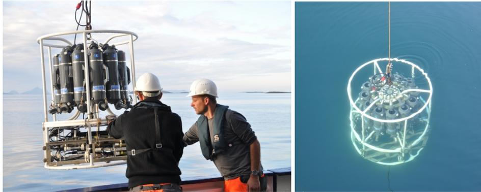
**Figure 1** Onboard device Seabird 'sbe911+' CTD probe with sampling rosette at station work on *R/V Heincke*.
