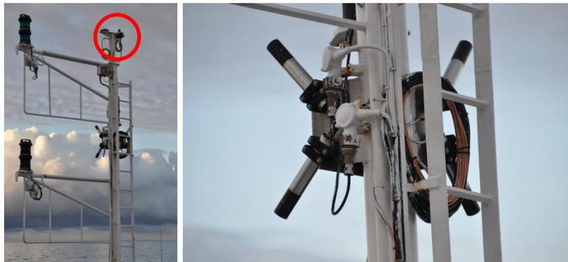
**Figure 6** Radiometric set-up on the foremast of R/V Heincke. One RAMSES-ACC hyperspectral cosine irradiance meter was installed at the top of the mast to measure total downwelling solar irradiance (red circle).
