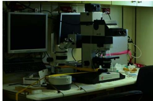
**Figure 7** Harvesting of surface plankton by vertical net tow (20  $\mu\text{m}$ -mesh) and subsequent analysis of net tow concentrate by stereo dissecting and phase interference (Nomarski) microscopy.
