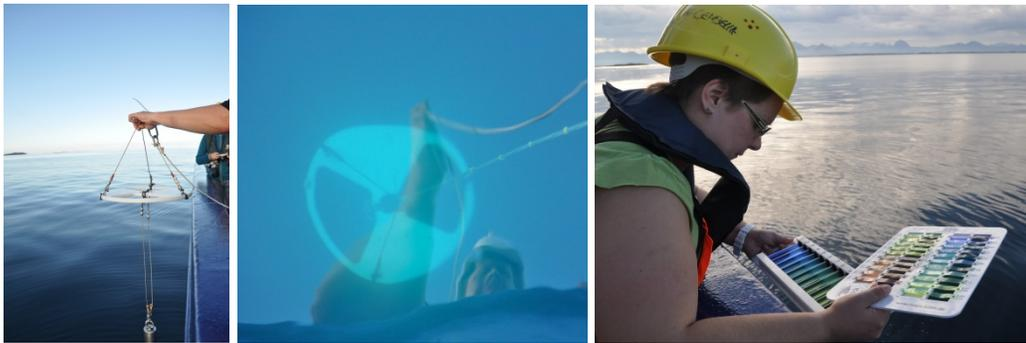
**Figure 5** Secchi disc above and in water (left, middle) and Forel-Ule (FU) color comparator scale to determine the water color (right).
