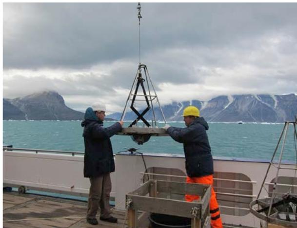
**Figure 10** Deploying a Van Veen sediment sampler near Disko Bay, Greenland, similar in design to that used to collect sediments from the Norwegian coast aboard *RV Heincke HE431*.
