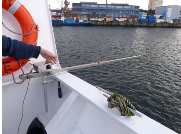
Figure 5: Device on R/V ALKOR for controlling the position of the sphere, similar to a fishing rod.
