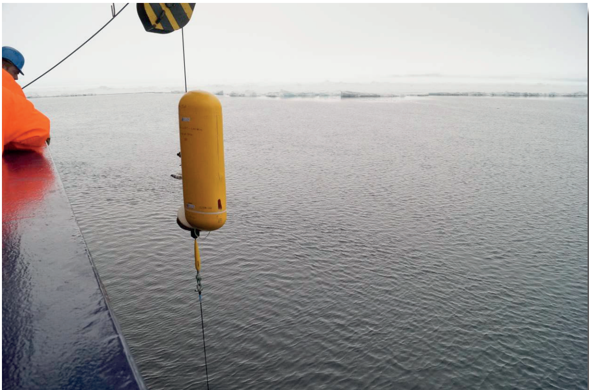
Fig. 8.3: Deployment MMP- profiler
