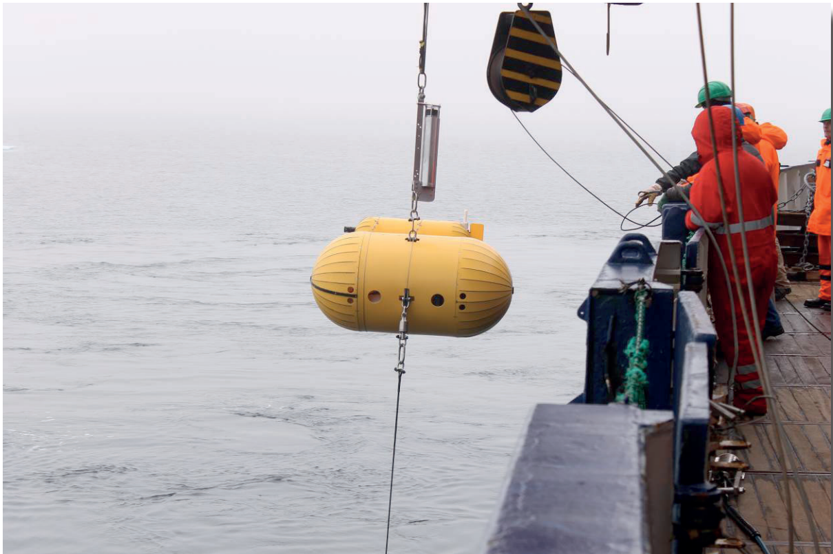
Fig. 8.2: Subsurface winch and profiler during deployment
