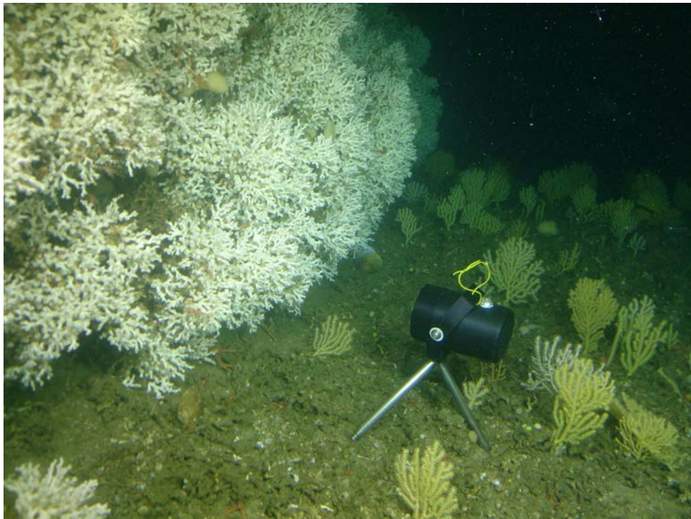
Figure 2 Underwater video camera system (version 2.0) placed in front of a whole L. pertusa colony. Nordleksa reef. (Photo: JAGO team).
