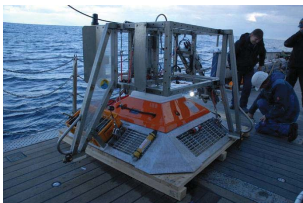
Fig. 4.3.1: Trawl resistant lander with launcher ready for deployment.
