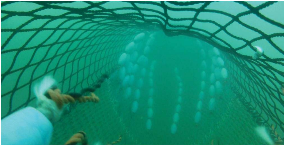
Figure 2: Screenshot from underwater recordings of codend with stimulation ropes
