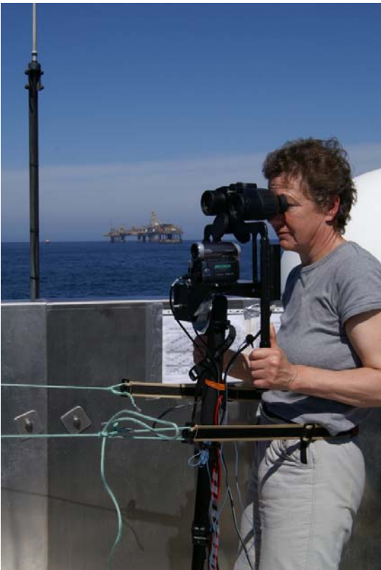
Figure 8: SCANS II – West Freezer: An easily ‘designed’ and well performing safety sling for the 7x50 tracker
