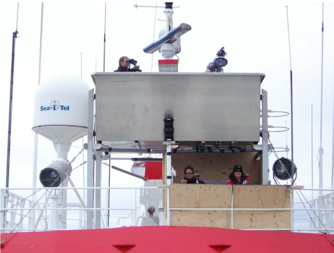
Figure 4. SCANS II – West Freezer: Special anti-vibrating mounting of the tracker platform
